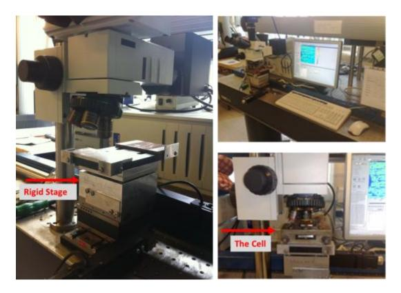
Figure: 3-9: Setup of the rig under the DIC optical microscope.
