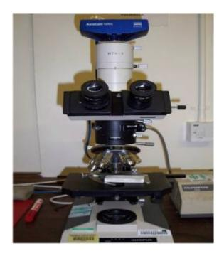
Figure 3-15: Optical Microscope (OM), Olympus-BH2.
