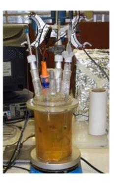
Figure 4-4: Change in the solution colour after testing samples in 30%NaCl at 80°C, pH=5.8, half cycle polarisation test shown in Figure 4-3.
