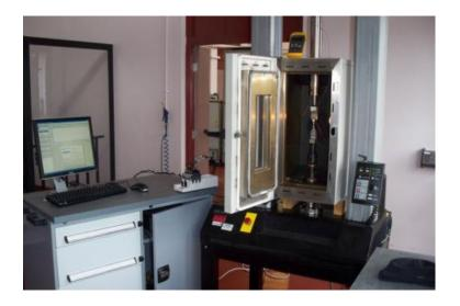
Figure 3-8: Mechanical tensile testing machine INSTRON 5569.
