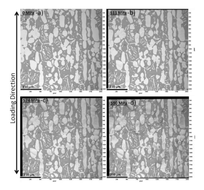
Figure 4-81: Optical micrographs captured at four different strain levels of a) No Stress, b) at 511 MPa -1% Strain, c) at 574 MPa – 2% Strain and d) at 590 MPa -3% Strain (ferrite is dark and austenite is light).
