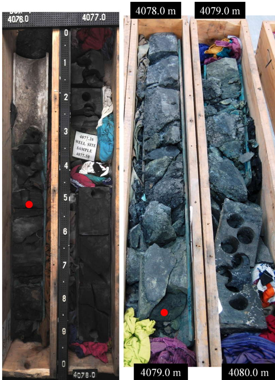
Figure 13. Depth interval from 4076.3-4076.5 m represents brecciated mudstones (LF8), from 4076.5.0-4077.6 m represents laminated microcrystalline quartz-rich, detritus-bearing mudstones (LF3) and from 4077.6-4080.0 m represents either slumped mudstones (LF7) or LF8. The red circles show core depth of the thin-section microphotographs presented in Figure 14. These samples are (from top to bottom): ALNR-2(25) and ALNR-2(26).
