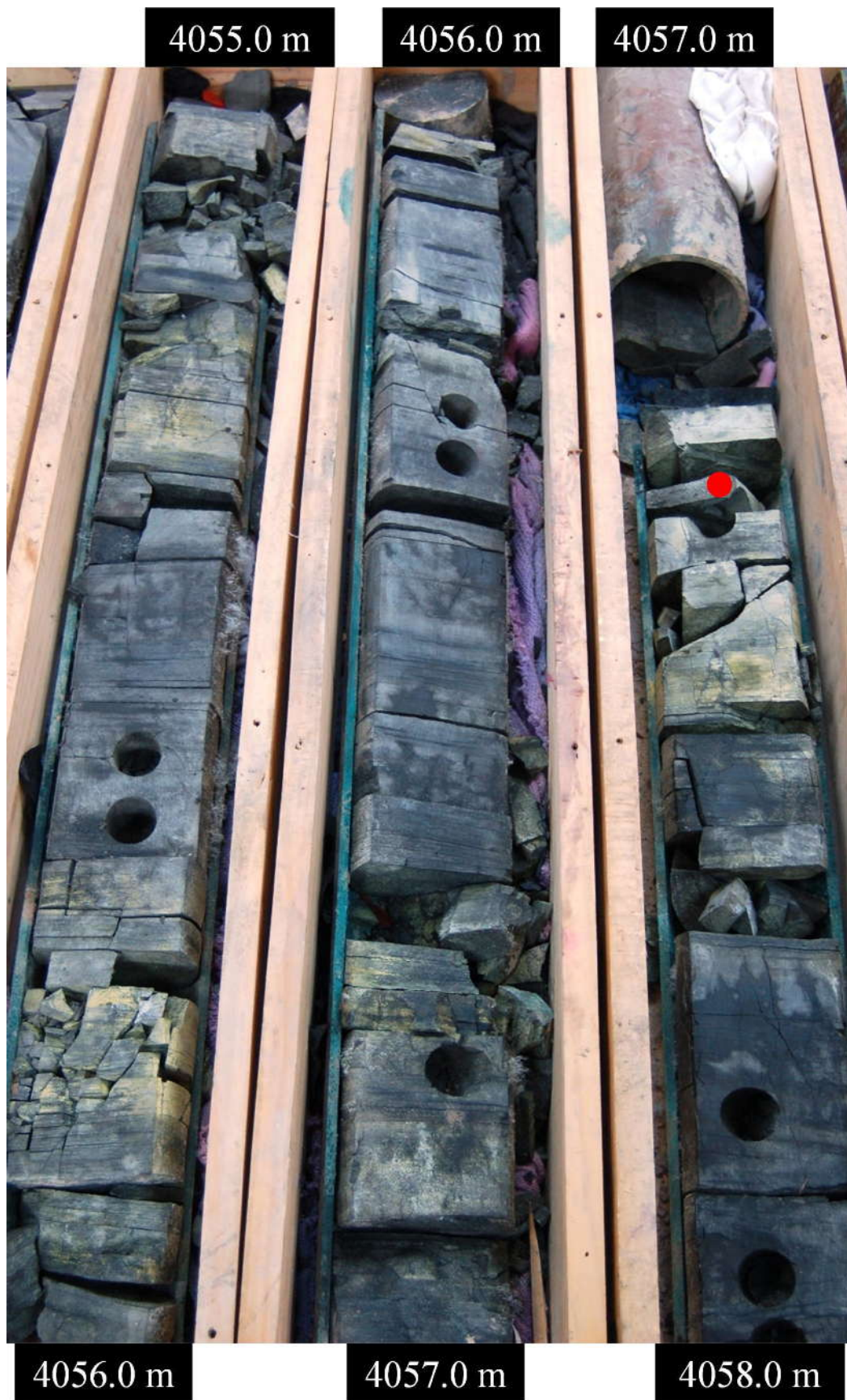
Figure 7. Depth interval from 4055.0-4058.0 m represents laminated microcrystalline quartz-rich, detritus-bearing mudstones (LF3), which is moderately fissile and laminated. The red circle shows core depth of the thin-section microphotographs of sample ALNR-2(15) presented in Figure 9.
