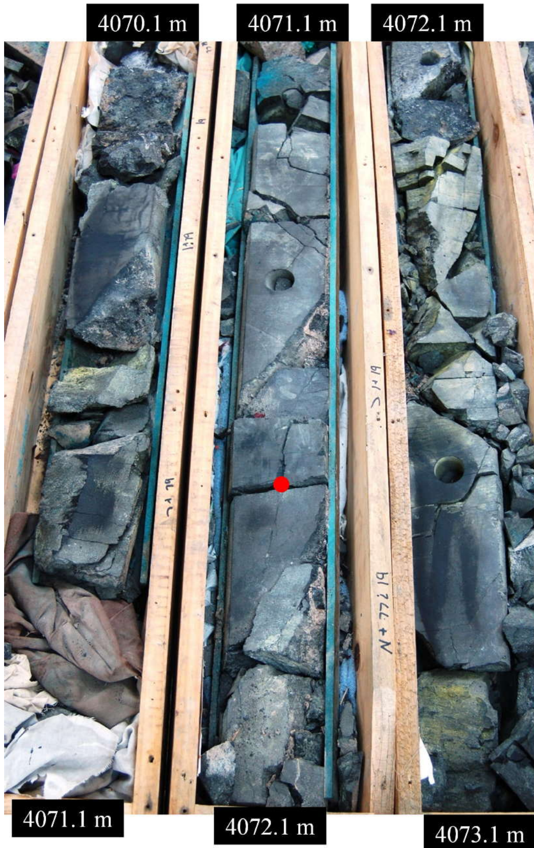
Figure 12. Depth interval from 4070.1-4070.2 m represents brecciated mudstones (LF8), from 4070.2-4073.1 m represents laminated microcrystalline quartz-rich, detritus-bearing mudstones (LF3). The red circle shows core depth of the thin-section microphotographs of sample ALNR-2(24) presented in Figure 14.
