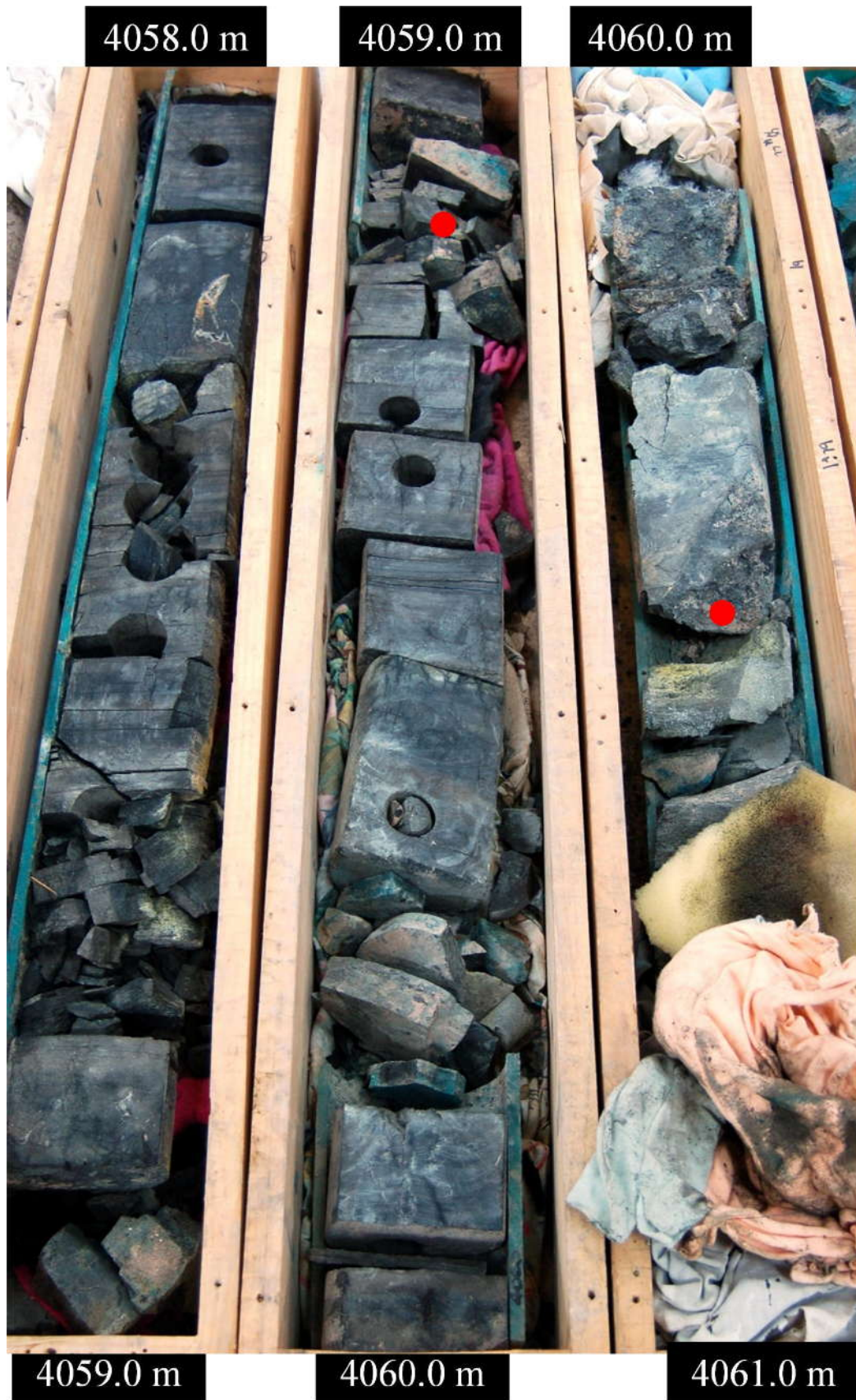
Figure 8. Depth interval from 4058.0-4060.0 m represents laminated microcrystalline quartz-rich, detritus-bearing mudstones (LF3), from 4060.0-4060.25 m represents slumped mudstones (LF7) and from 4060.25-4060.75 m represents LF3. The red circles show core depth of the thin-section microphotographs presented in Figure 9. These samples are (from top to bottom): ALNR-2(16) and ALNR-2(17).
