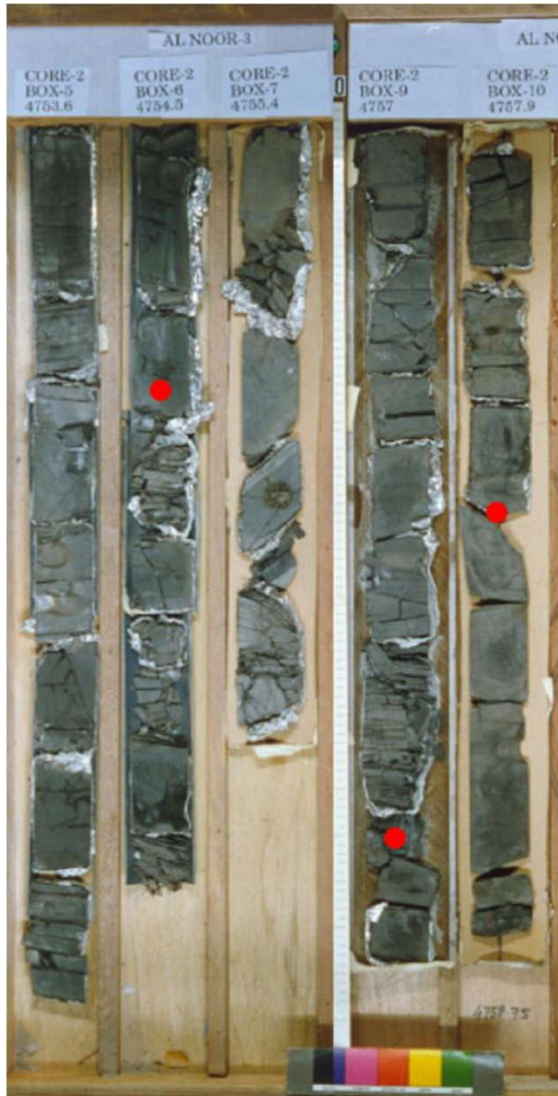
Figure 22. Depth interval from 4753.6–4754.7 m represents laminated microcrystalline quartz-rich, detritus-bearing mudstones (LF3), from 4754.7–4754.9 m represents laminated microcrystalline quartz-dominated mudstones (LF2), from 4754.9–4756.0 m represents alternation between laminated microcrystalline quartz-rich mudstones (LF1; highly fissile) and LF3 (moderately fissile) in 0.1 m scale, from 4757.0 to 4758.75 m represents mainly LF3 apart from thin interval from 4757.6–4757.8 that represents LF1 (fissile and strongly laminated). The red circles show core depth of the thin-section microphotographs presented in Figures 23. These samples are (from top to bottom): ALNR-3(9), ALNR-3(11) and ALNR-3(12).
