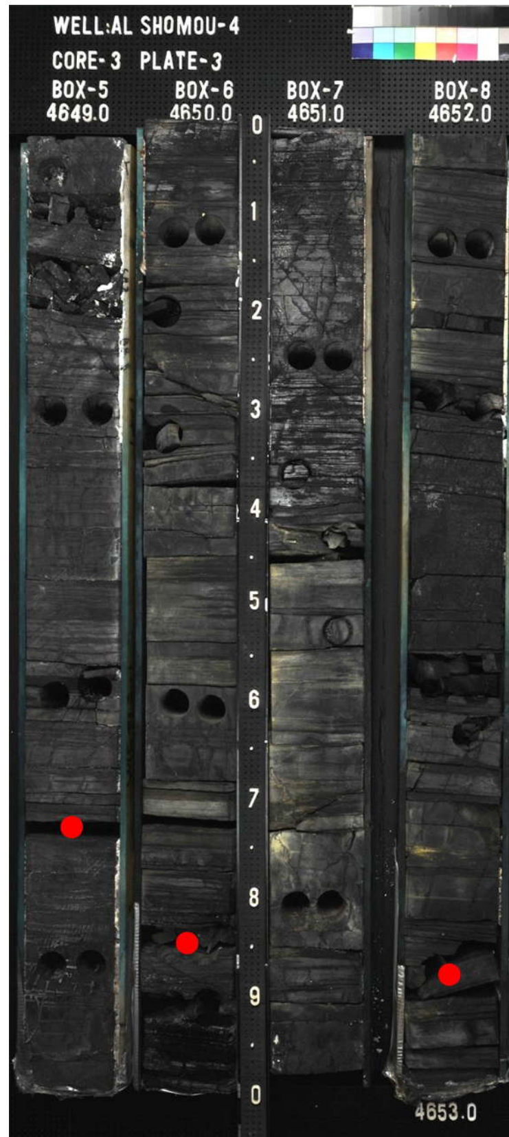
Figure 34. Depth interval from 4649.0-4650.45 m represents laminated microcrystalline quartz-rich mudstones (LF1), from 4650.45-4651.0 m represents laminated microcrystalline quartz-rich, detritus-bearing mudstones (LF3), from 4651.0-4651.45 m represents LF1, and from 4651.45-4653.0 m represents LF3. The red circles show core depth of the thin-section microphotographs presented in Figures 35. These samples are (from top to bottom): ASH-4(16), ASH-4(17) and ASH-4(20).
