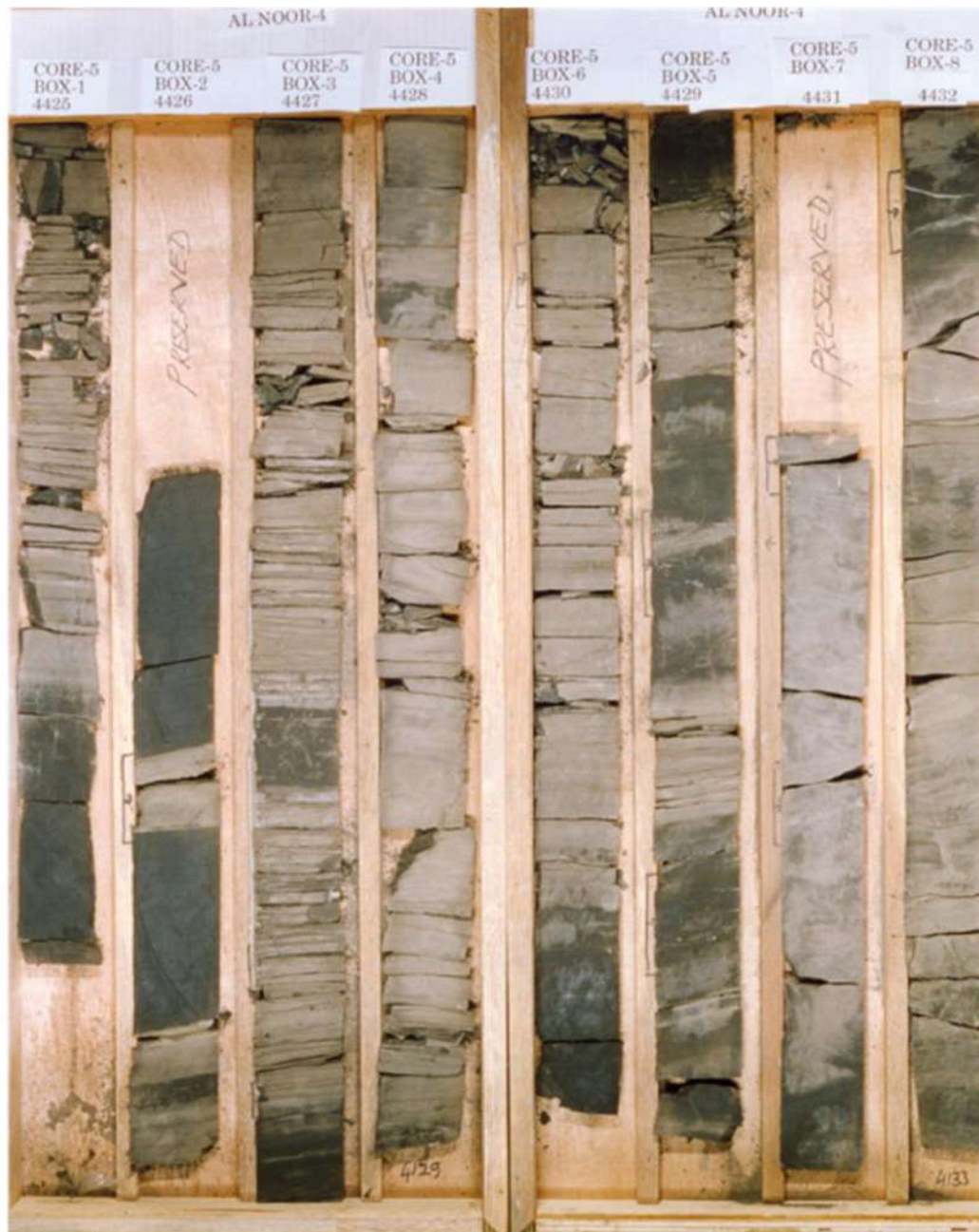
Figure 26. Depth interval from 4425.0-4433.0 m represents alternation between laminated microcrystalline quartz-rich mudstones (LF1) and laminated microcrystalline quartz-dominated mudstones (LF2). LF1 is very fissile and well-laminated, while LF2 is dark-coloured, not fissile and show very weak lamination.
