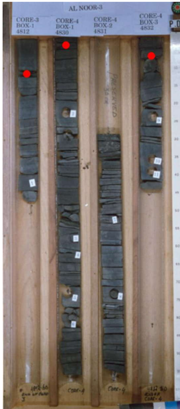
Figure 24. Depth interval from 4812.0-4812.6 m represents either laminated microcrystalline quartz-rich mudstones (LF1) or laminated microcrystalline quartz-rich, detritus-bearing mudstones (LF3; very hard to distinguish from the core, but the sample obtained from this depth suggests that this interval represents LF1), from 4830.0-4832.3 m represents LF1, from 4832.3-4832.5 m represents laminated microcrystalline quartz-dominated mudstones (LF2). The red circles show core depth of the thin-section microphotographs presented in Figures 25. These samples are (from top to bottom): ALNR-3(13), ALNR-3(14) and ALNR-3(15).
