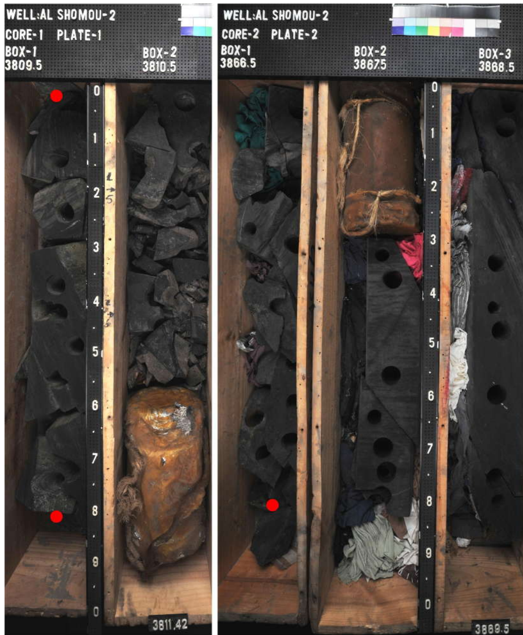
Figure 28. Depth interval from 3809.5-3810.6 m and from 3866.5-3869.5 m might represent either laminated microcrystalline quartz-dominated mudstones (LF2) or laminated microcrystalline quartz-rich, detritus-bearing mudstones (LF3). Microscopic analysis of the samples obtain from these intervals suggest that interval from interval from 3809.5-3810.6 m represents laminated microcrystalline quartz-rich mudstones (LF1) and LF3 and depth interval from 3866.5-3869.5 m represents LF3. The red circles show core depth of the thin-section microphotographs presented in Figures 29. These samples are (from top to bottom): ASH-2(1), ASH-2(2) and ASH-2(4).
