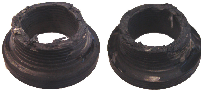
Figure 7.7: Typical failed cylindrical specimen
