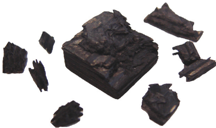
Figure 7.8: Typical failed cube specimen
