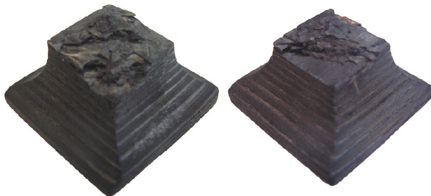
Figure 7.6: Typical failed waisted specimen
