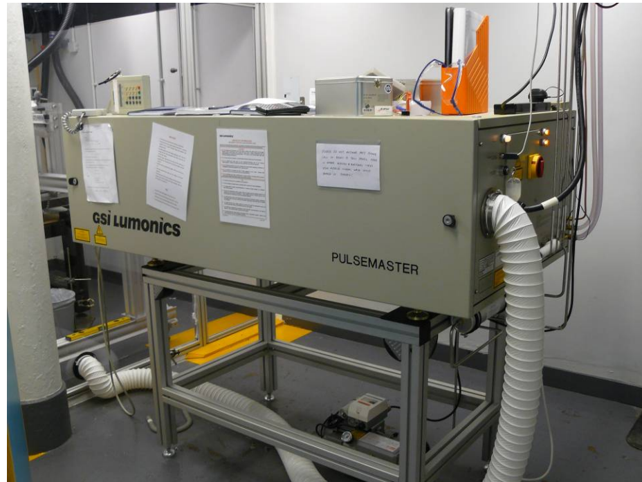
Figure 4-8: The KrF excimer laser used to irradiate various spin-coated and as-dried \text{TiO}_2 films on glass
