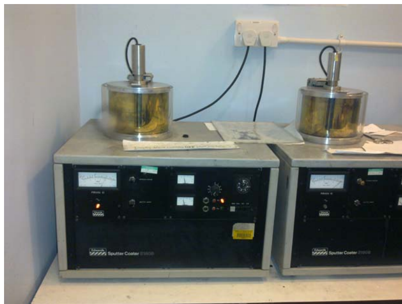
Figure 4-19: A gold sputtering unit used for the conductive coating of the \text{TiO}_2 films
