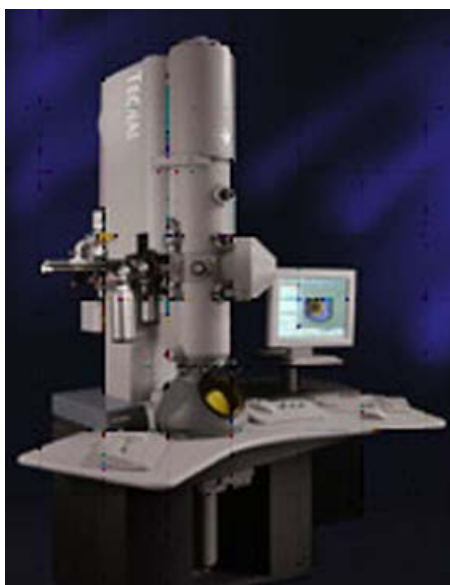
Figure 4-20: Tecnai F30 STEM used to investigate various TiO 2 films
