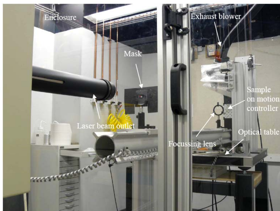
Figure 4-10: Photograph of a typical laser setup used to prepare various TiO 2 -based films by SGLIT
