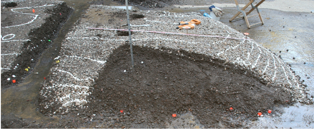
Figure 17. Photograph of the 27th August deposit termination. Approximately 5 cm of surface material has been removed from a sector of the deposit, uncovering two white tracer stones. The surface material removed, like that visible behind the excavated sector, is strongly coarse-enriched. White lines on the undisturbed deposit surface are topographic contours, determined by laser leveling and applied with paste.
