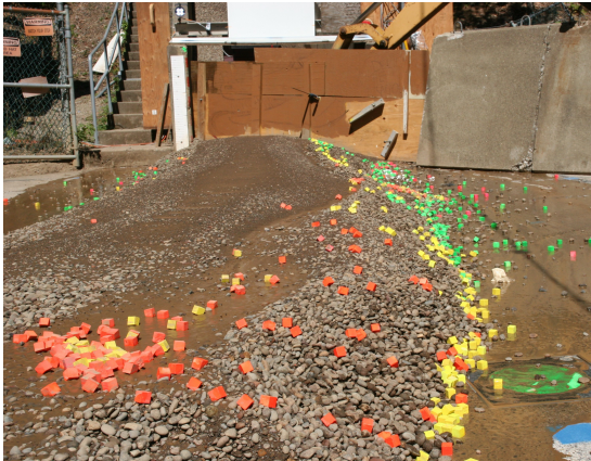
Figure 7. Oblique ground-level photograph of the August 25th experimental deposit, looking upslope from the deposit termination. Tracer cubes deposited on the surface lie on or near the levee walls at the flow margins, rather than in the central channel. The tracer cubes are deposited in coloured bands, from orange cubes near the deposit termination (foreground), then yellow, then green, then pink cubes near the flume mouth. This pattern represents a reversal of the order in which the cubes were seeded onto the flow surface; the last cubes to be seeded onto the flow (orange), were deposited furthest from the flume mouth.
