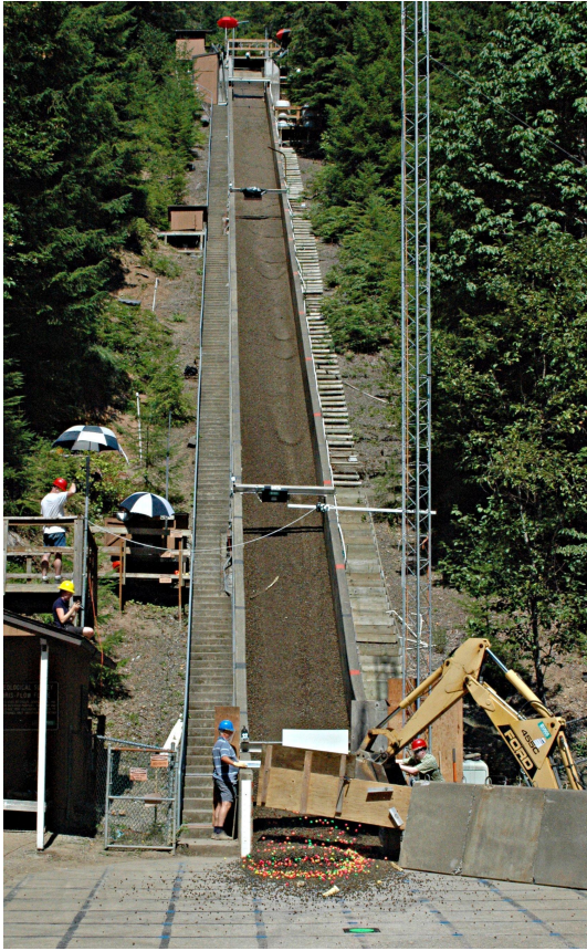
Figure 1. The USGS debris-flow flume, near Blue River, Oregon. This photo shows a debris flow \sim 14 s after it has been released from the hopper (top centre). The head of the debris-flow has reached the runout pad at the bottom of the flume, and has coloured tracers on its surface which were dropped onto it as the flow exited the flume mouth. A wooden barricade, held above the flume mouth with the back-hoe of a tractor, allows the initial stages of the debris flow runout to pass beneath it unimpeded. The barricade is dropped across the flume mouth once the bulk of the flow has passed, diverting the watery flow ‘tail’.
