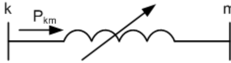
Figure 7.9: the variable series reactance model of TCSC.
