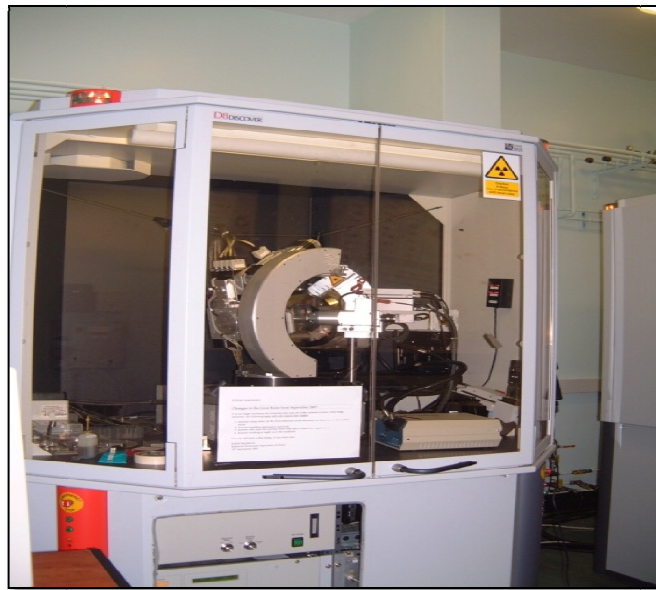
Figure 4.13: The Bruker AXS D8 Discover laboratory X-ray diffractometer configured for stress measurement
