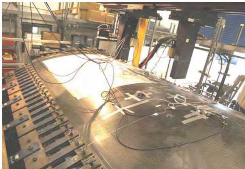
Figure 2.11 Composite structure with acoustic emission sensors [4]
