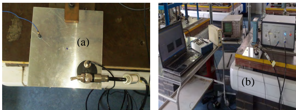
Figure 3.1 Schematic of Experiments, (a) Plate with shaker and accelerometer, (b) Experimental setup
