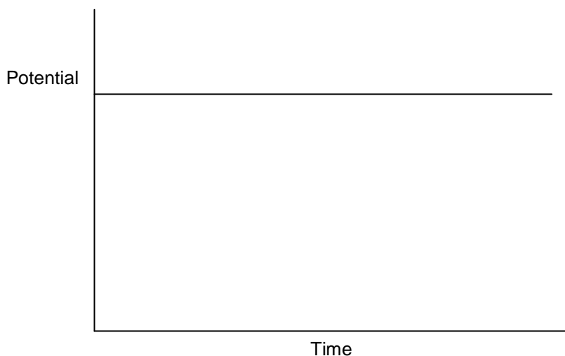
Figure 2.11 Typical waveform for amperometry in stirred solution
