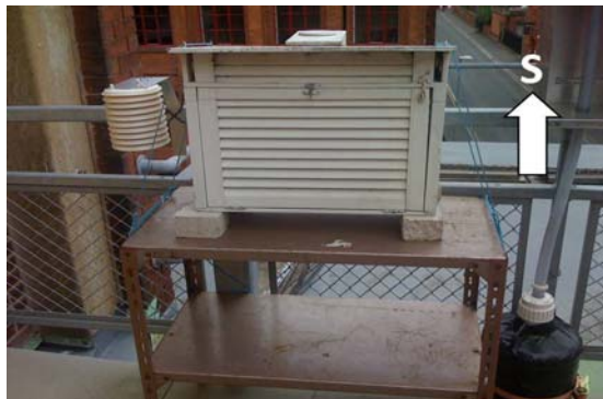
Figure 5.13 Orientation of Stevenson Screen and radiation shield (white arrow points South)
