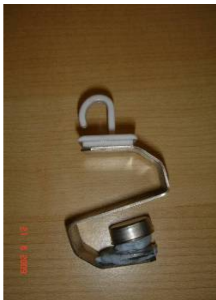
Figure 5.5 Typical hook design with sensor-logger
