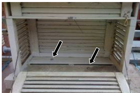
Figure 5.12 Sensor-logger locations inside Stevenson Screen
