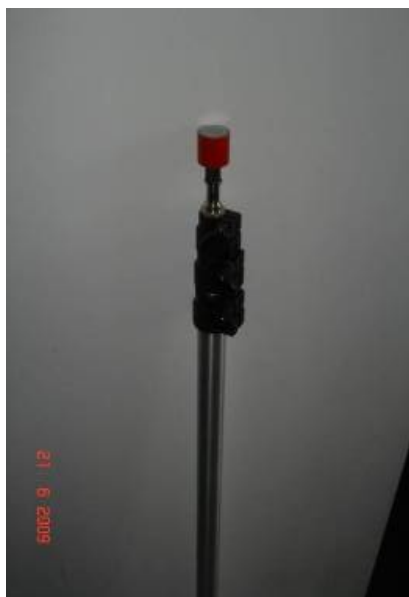
Figure 5.4 Telescopic rod used to hang sensor-logger
