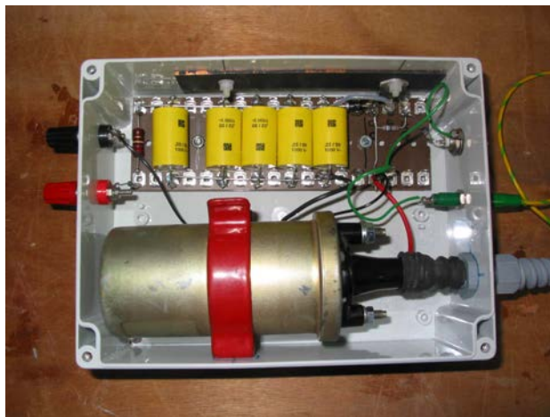
Figure 4.5: The completed 20kV spark generator
