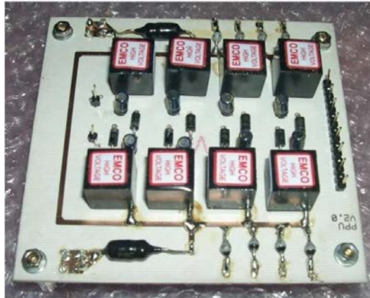
Figure 6.10: Revised PPU developed during bread boarding for the STRaND-1 CubeSat
