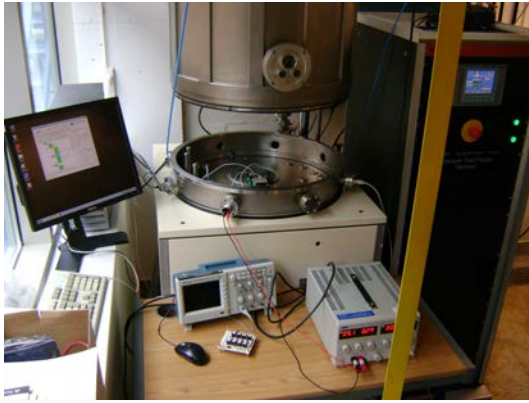
Figure 6.19: Left: Qualification model in the vacuum chamber discharging. Right: Voltage discharge profile across the capacitor terminals
