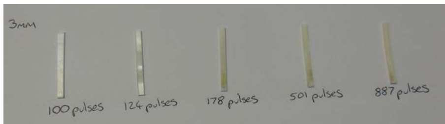
Figure 4.25: Carbon build up on the Teflon TM samples as a function of total number of pulses
