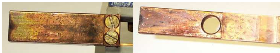
Figure 4.35: The electrode surfaces after exposure to several thousand pulse discharges at various energies. Left: Anode, Right: Cathode, the hole is the location of the sparkplug insert
