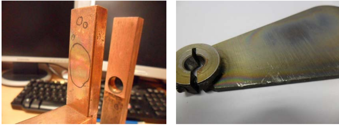
Figure 4.37: Examples of film deposition Left: Back of PPT anode, Right: surface of metal flange from a plasma deposition chamber
