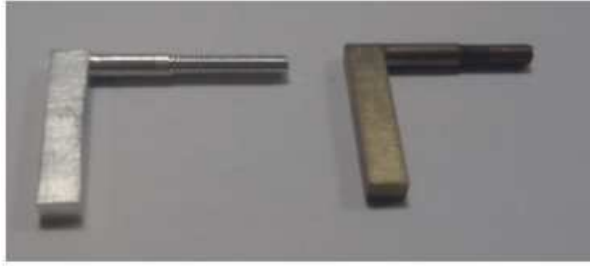
Figure 6.5: Contact arms. Left: Aluminium, Right: Elkonite
