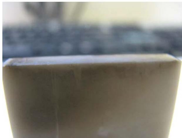
Figure 4.17: Carbon build up on the Teflon TM surface
