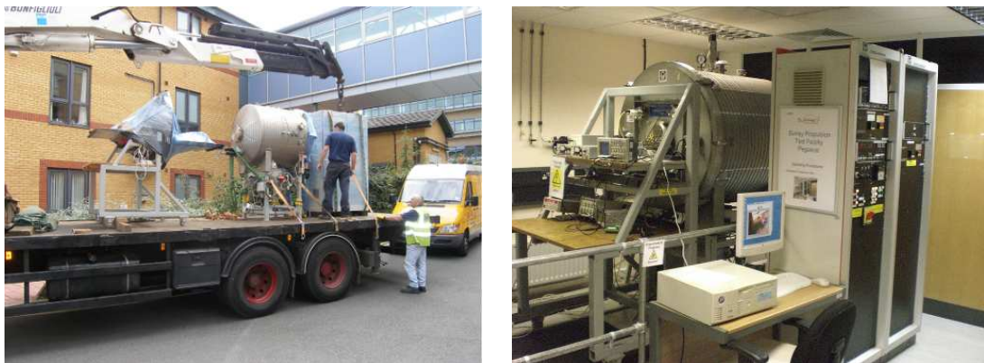
Figure 4.9: Left: Moving of the large vacuum chamber from Astrium to the Surrey Space Centre. Right: The chamber in its original configuration
