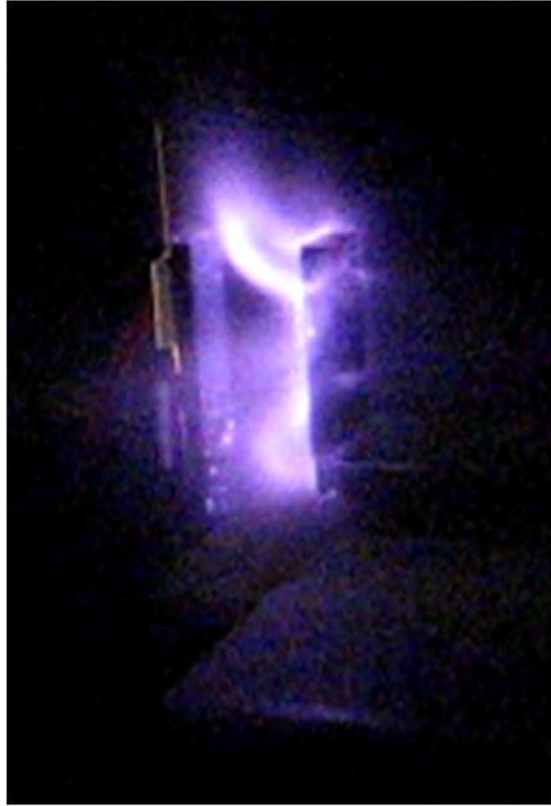
Figure 4.19: A still image of the plasma forming during a PPT discharge without Teflon TM propellant
