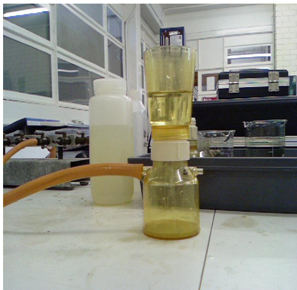
Photo 4.11 Filtration unit 0.45 µm membrane filter
