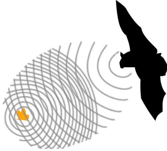
Figure 2.15- Waves propagate from the bat in the direction of the prey target, where a reflected echo occurs.
