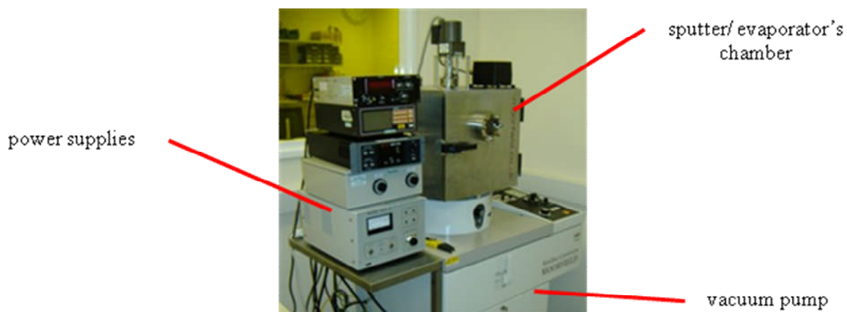
Figure 4.5 The Moorfield sputter/evaporator used for metal deposition applications without breaking the vacuum.
