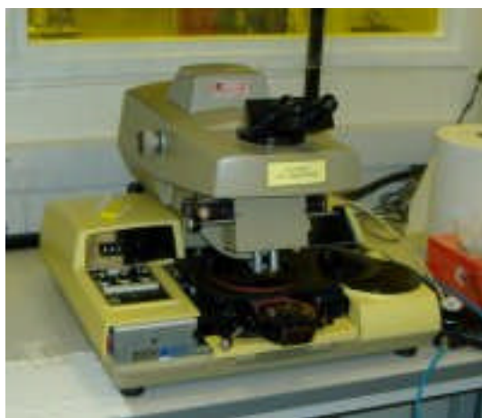
Figure 4.4 The CA-800 mask aligner, using a 200 Watt UV mercury short-arc exposure system (exposure uniformity \sim 5\% over 4\frac{1}{2} - inch diameter area) used for sample patterning.
