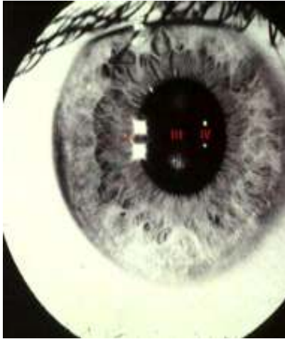
Figure 6.2 Purkinje reflections, from the cornea (I) and crystalline lens (III and IV). Digital eye trace made use of the corneal image only.
