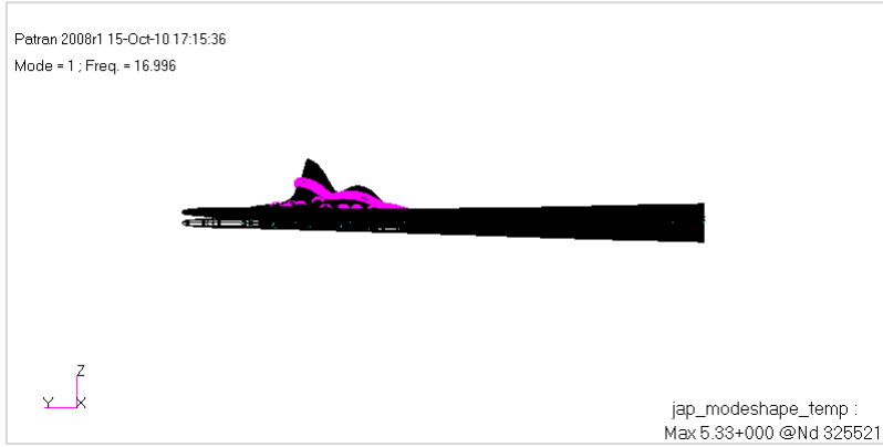
First Bending ; 16.9 Hz
