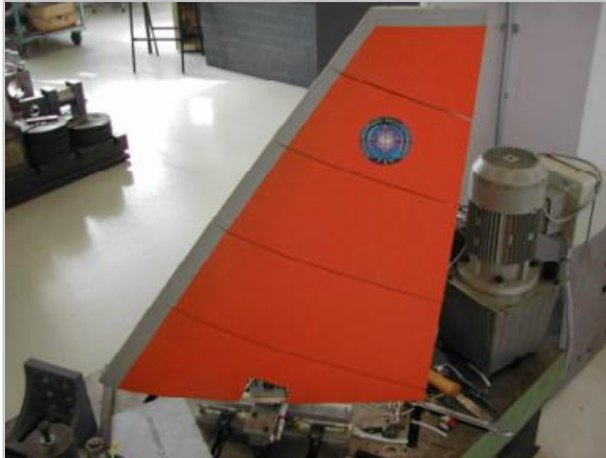
Figure 2.8 All Movable Vertical Tail (AMVT) with Variable Stiffness Attachment [29]
