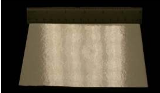
Photograph of impact damage coupon #30 (17ply + mesh painted, Ø87mm/40J)
