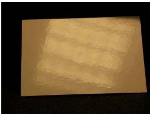
Photograph of impact damage coupon #94 (17ply + mesh painted, Ø87mm/10J)
