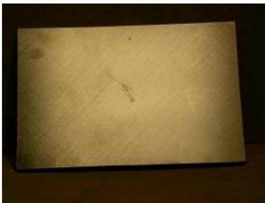
Photograph of impact damage coupon #U57 (33ply unpainted, tool shape/30J)
