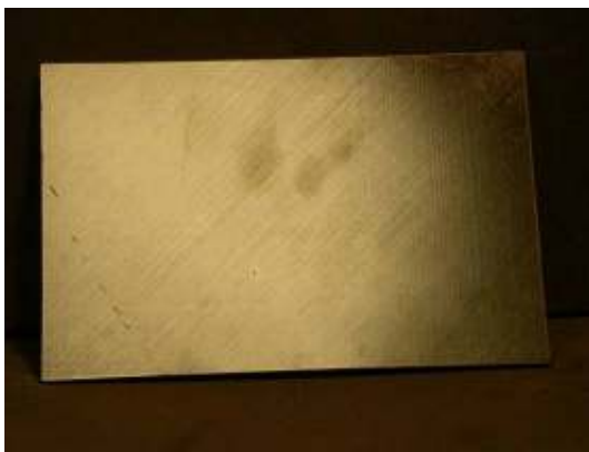
Photograph of impact damage coupon # U23 (17ply unpainted, Ø87mm/40J)
