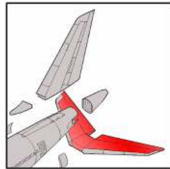
Figure 2.03 – Detail of Horizontal Stabiliser Courtesy of Airbus
