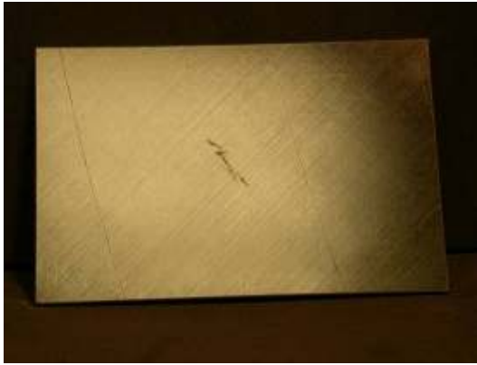
Photograph of impact damage coupon #U32 (17ply unpainted, tool shape/15J)
