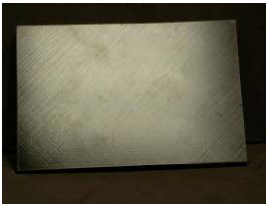
Photograph of impact damage coupon #U38 (33ply unpainted, Ø20mm/5J)
