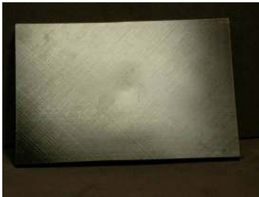
Photograph of impact damage coupon #U49 (33ply unpainted, Ø87mm/70J)
