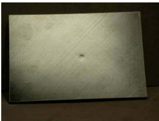
Photograph of impact damage coupon #U39 (33ply unpainted, Ø20mm/10J)
