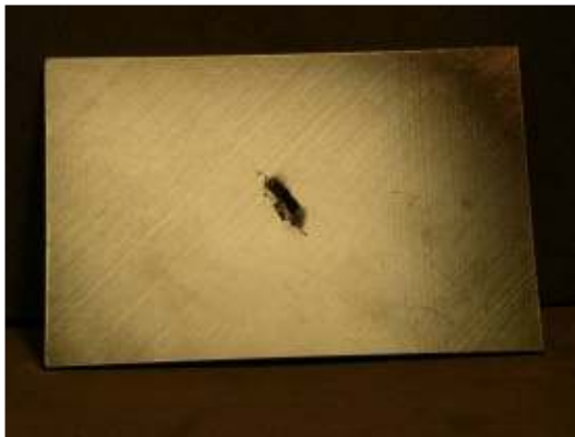
Photograph of impact damage coupon #U34 (17ply unpainted, tool shape/17.5J)
