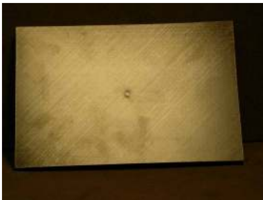
Photograph of impact damage coupon #U42 (33ply unpainted, Ø20mm/30J)
