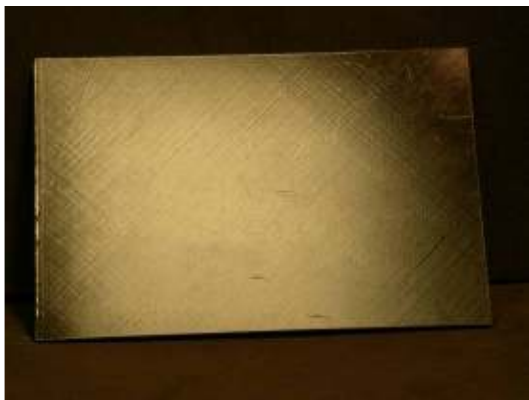
Photograph of impact damage coupon #U30 (17ply unpainted, tool shape/5J)
