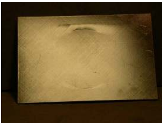
Photograph of impact damage coupon #U29 (17ply unpainted, Ø70mm cylinder/40J)
