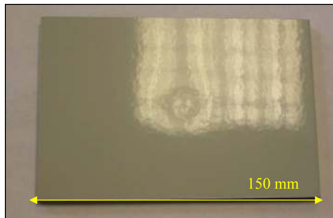
Figure 4.16 – Impact damage surface flaw on a painted/ bronze mesh CFRP laminate
