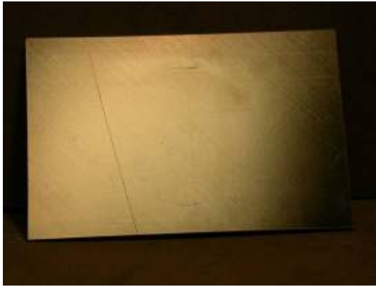
Photograph of impact damage coupon #U27 (17ply unpainted, Ø70mm cylinder/20J)
