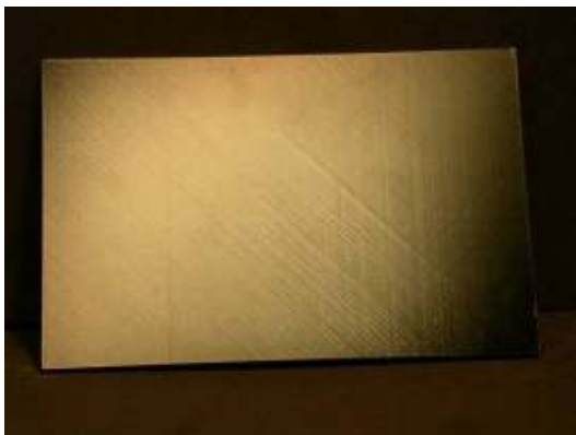
Photograph of impact damage coupon #U18 (17ply unpainted, Ø87mm/5J)
