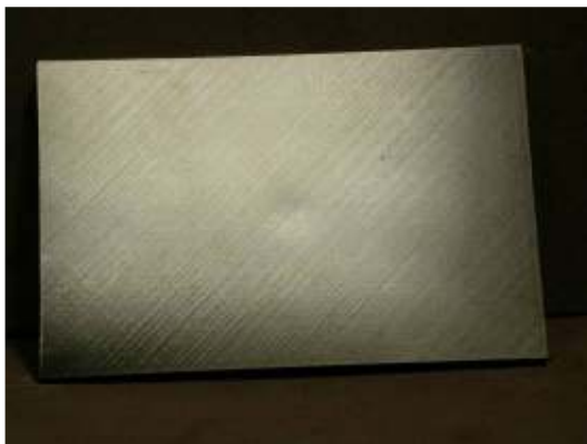
Photograph of impact damage coupon #U44 (33ply unpainted, Ø87mm/20J)
