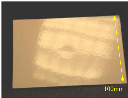
Figure 5.11 - surface flaw produced by 30J / Ø87 mm impact on 17ply painted laminate
