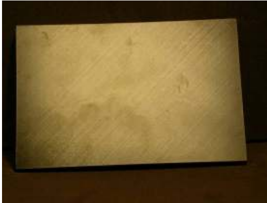
Photograph of impact damage coupon #U51 (33ply unpainted, Ø70mm cylinder/20J)
