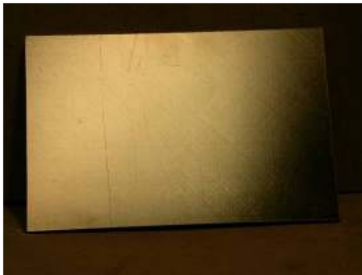
Photograph of impact damage coupon #U25 (17ply unpainted, Ø70mm cylinder/10J)
