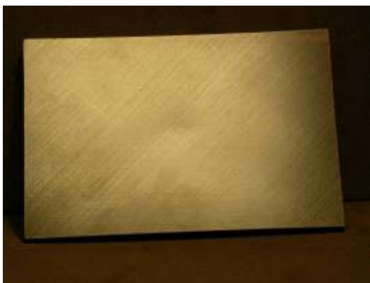
Photograph of impact damage coupon #U47 (33ply unpainted, Ø87mm/50J)
