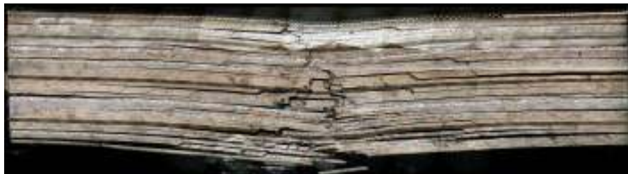
Metallographic section image of Ø20mm/50J impact (from Boulic, 2007)
