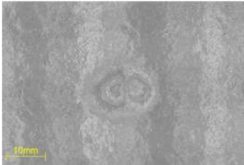
Figure 5.07 – 15J / Ø20 mm impact on 17ply painted laminate
