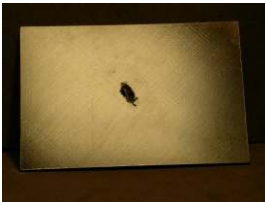
Photograph of impact damage coupon #U35 (17ply unpainted, tool shape/20J)
