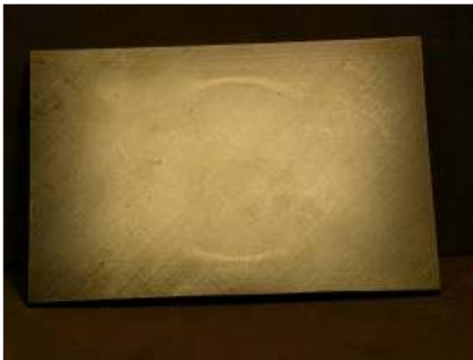
Photograph of impact damage coupon #U55 (33ply unpainted, Ø70mm cylinder/60J)
