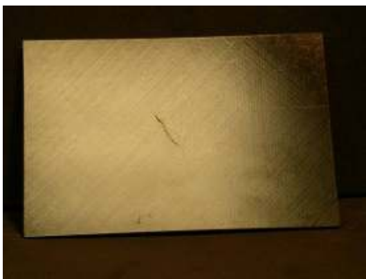
Photograph of impact damage coupon #U31 (17ply unpainted, tool shape/10J)
