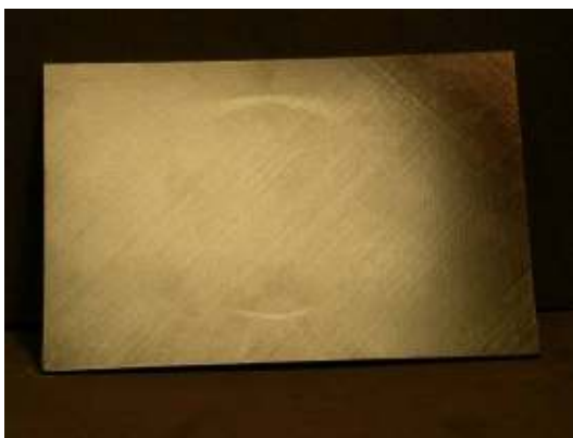
Photograph of impact damage coupon #U26 (17ply unpainted, Ø70mm cylinder/15J)
