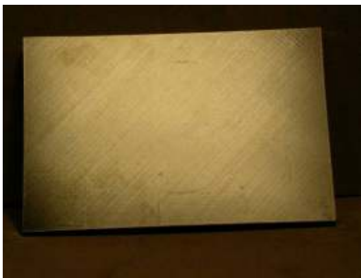
Photograph of impact damage coupon #U52 (33ply unpainted, Ø70mm cylinder/30J)
