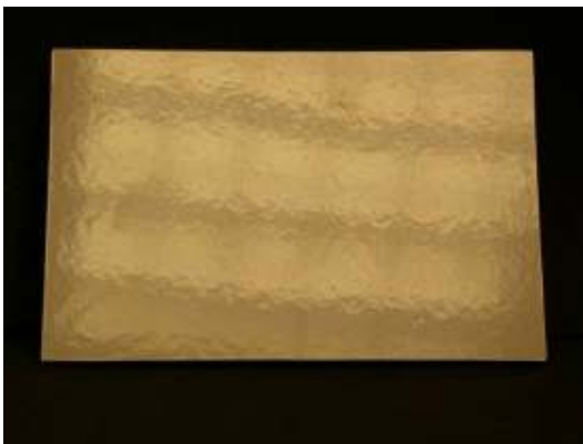
Photograph of impact damage coupon #34 (17ply + mesh painted, tool shape/5J)
