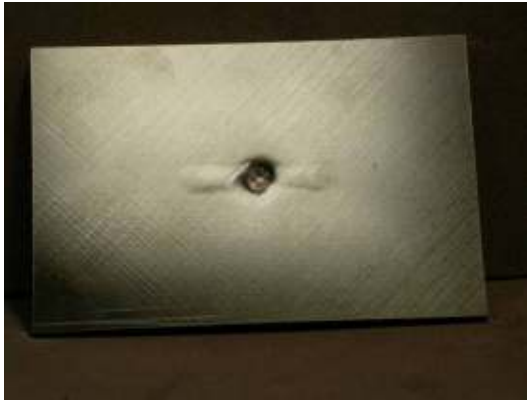
Photograph of impact damage coupon #U43 (33ply unpainted, Ø20mm/50J)
