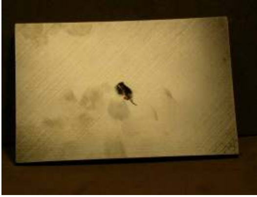
Photograph of impact damage coupon #U59 (33ply unpainted, tool shape/50J)
