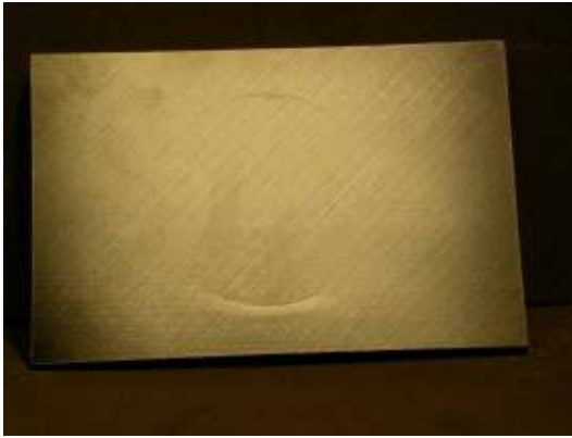
Photograph of impact damage coupon #U54 (33ply unpainted, Ø70mm cylinder/50J)
