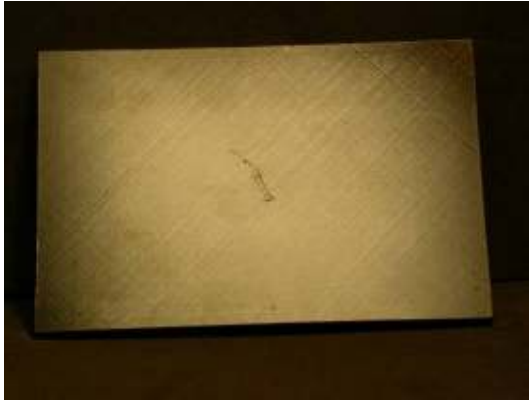
Photograph of impact damage coupon #U56 (33ply unpainted, tool shape/20J)
