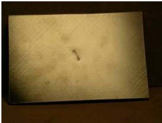
Photograph of impact damage coupon #U58 (33ply unpainted, tool shape/40J)
