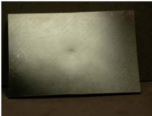
Photograph of impact damage coupon #U46 (33ply unpainted, Ø87mm/40J)
