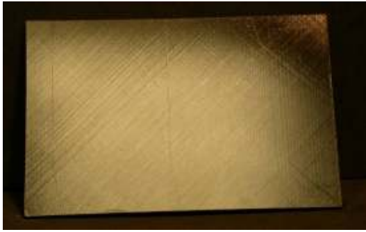
Photograph of impact damage coupon # U19 (17ply unpainted, Ø87mm/10J)
