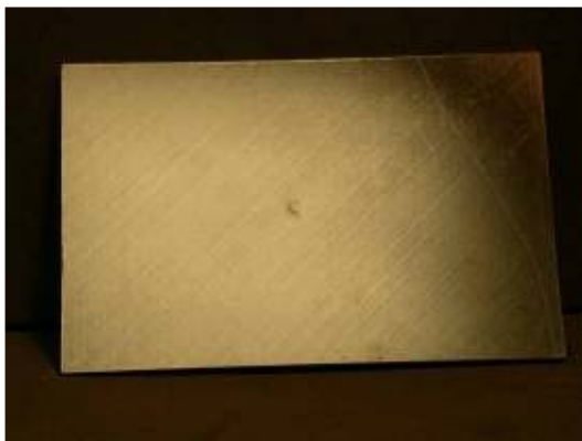
Photograph of impact damage coupon #U14 (17ply unpainted, Ø20mm/10J)
