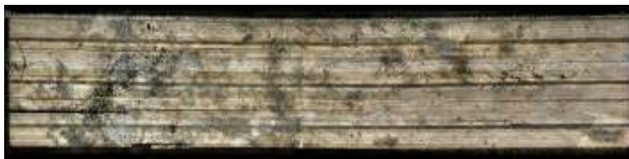
Metallographic section image of Ø87mm/60J impact (from Boulic, 2007)
