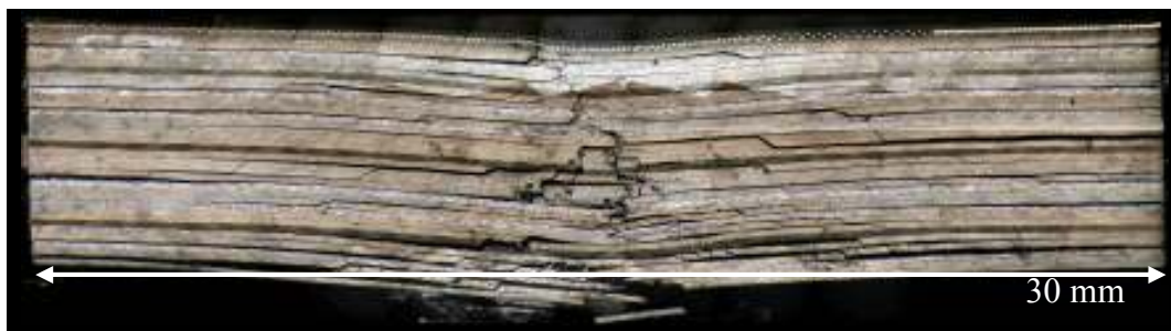
Figure 4.10 – Section through 50J, Ø20 mm impact on 33ply painted, mesh covered laminate
