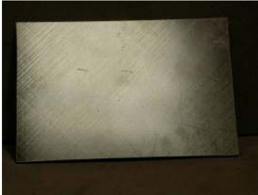
Photograph of impact damage coupon # U22 (17ply unpainted, Ø87mm/30J)
