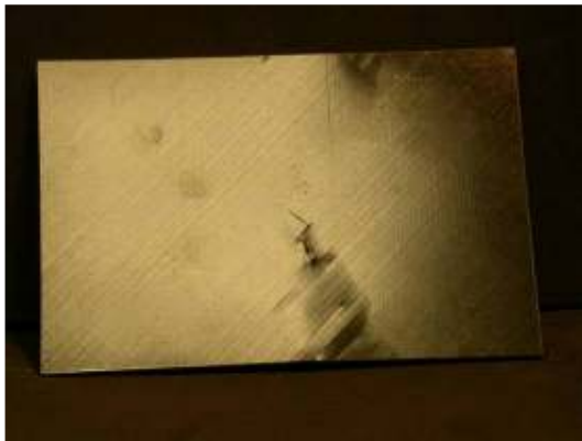
Photograph of impact damage coupon # U24 (17ply unpainted, Ø87mm/50J)
