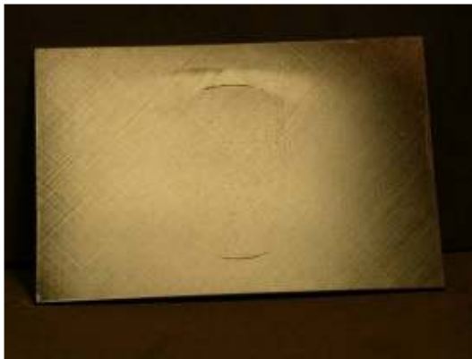
Photograph of impact damage coupon #U28 (17ply unpainted, Ø70mm cylinder/30J)
