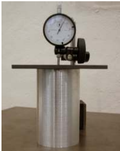
Figure 4.04 – Dial gauge measurement of surface flaw depth
