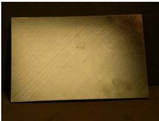
Photograph of impact damage coupon # U21 (17ply unpainted, Ø87mm/20J)
