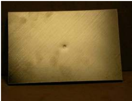
Photograph of impact damage coupon #U41 (33ply unpainted, Ø20mm/20J)
