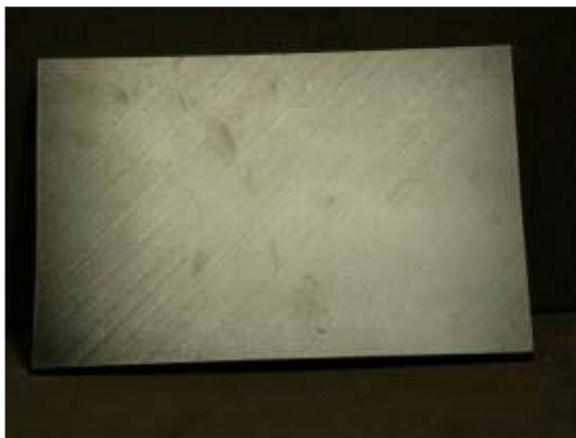
Photograph of impact damage coupon #U50 (33ply unpainted, Ø70mm cylinder/10J)
