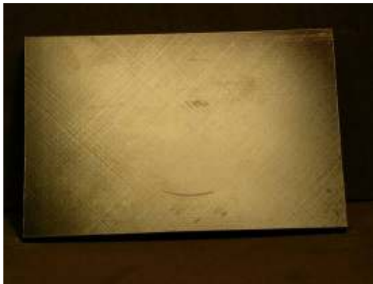
Photograph of impact damage coupon #U53 (33ply unpainted, Ø70mm cylinder/40J)
