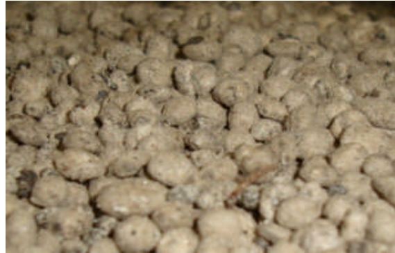
Figure 3.13: A sample of OMF 15 produced after coating biosolids granules sprayed with melted urea. Particle sizes in the range of 2.80 to 5.60 mm in diameter. [Picture facilitated by United Utilities plc].
