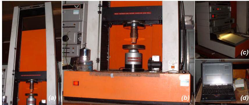
Figure 3.4: A picture showing the Instron 1122 (Instron, 1975); (a) overview of equipment, (b) close-up, (c) chart-drive system, and (d) laptop computer to record the measurements.
