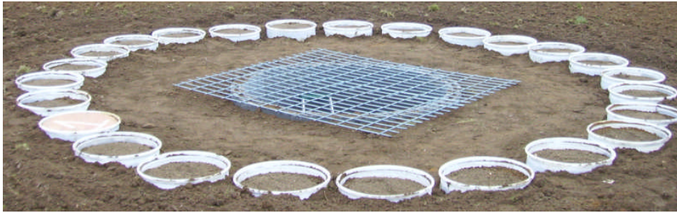
Figure 3: Overview of lysimeters' facility at Silsoe Farm following its construction in 2008.
