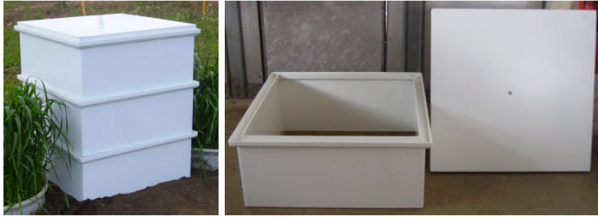
Figure 1.2: A picture showing the chambers used at the lysimeters station for measurement of N_2O emissions.
