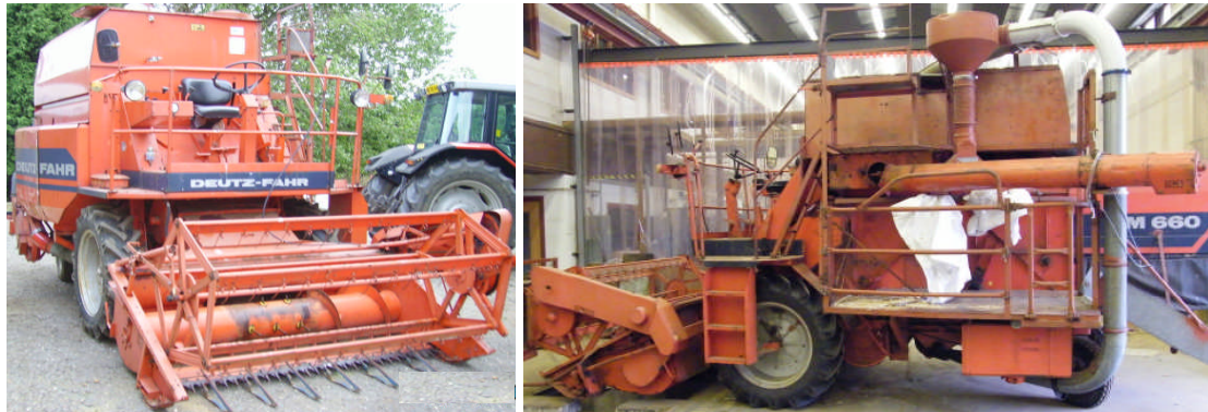
Figure A.7.6: Plot combine harvester Deutz-Fahr M660 used in the field experiments (left) and close-up of the bagging device (right).
