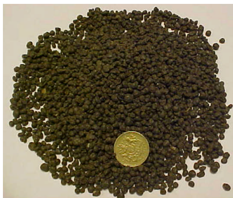
Figure 2: A picture showing OMF particles in the range 2 to 4 mm in diameter [Source: United Utilities plc].
