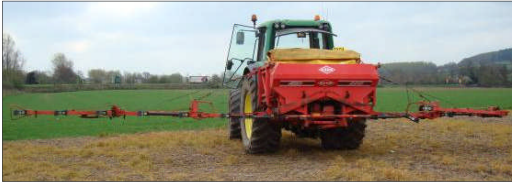
Figure 4.4: A picture showing the pneumatic spreading equipment used for the test.
