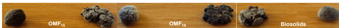
Figure 3.10: A picture of OMF 15 , OMF 10 and biosolids granules in the range of 3.35 to 4.00 mm in diameter showing the aspect of the particles before and after the compression test was conducted.
