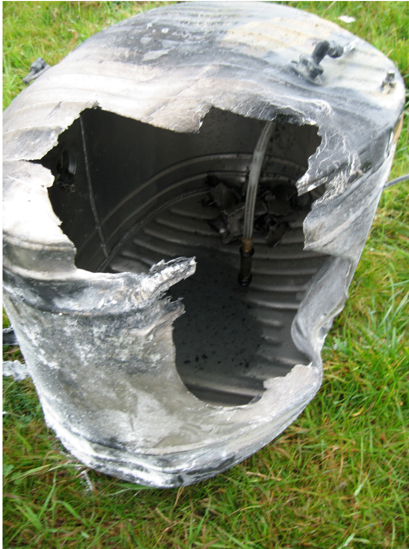
Figure 6.14: Fuel and tank deposits remaining in tank
