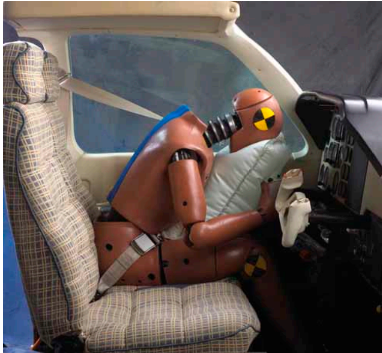
Figure 3.8: Seatbelt fitted airbag on general aviation aircraft Source: Amsafe, 2010
