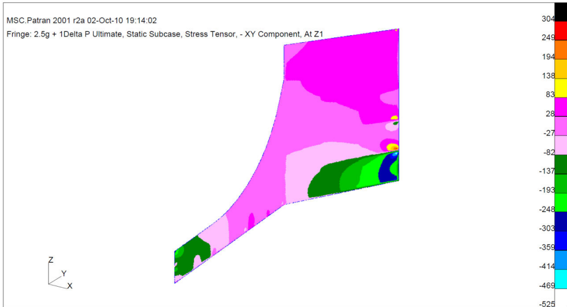
Figure 5.26 Shear stresses in spar
