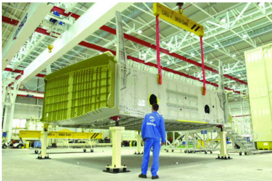
Figure 3.7 Picture of A380 centre box section (Flight International 2003)
