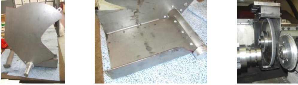
Figure 78 Extraction shroud featuring a) vacuum takeoff b) catchment plate c) clean machine
