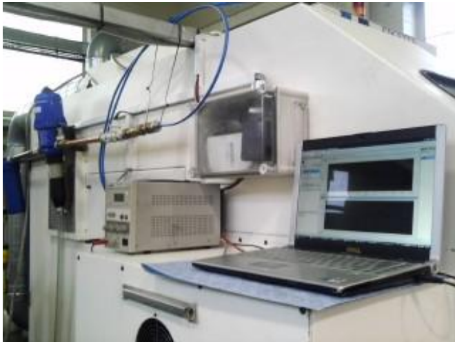
Figure 85 The machining fluid system in position. Water supply in from the rear of the machine under mains pressure. The Dosatron unit picks up the EcoCool oil from below before passing through sensors and fed directly to the nozzle through the side of the machine
