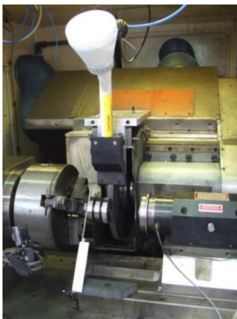
Figure 90 Design 3: Electrostatic Grinding Machine Setup. This set-up provided the lubricant to be applied by a pneumatic means, with or without the electrode being charged.
