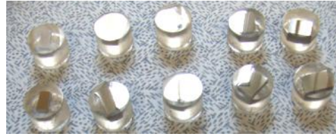
Figure 103 Finished samples. Embedded in resin body, polished and acid etched
