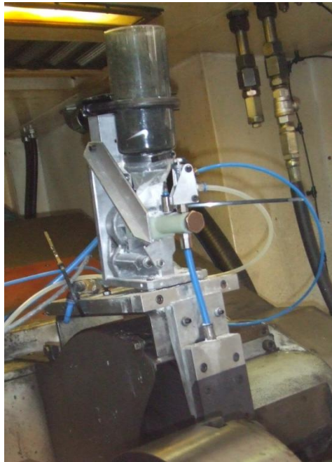
Figure 89 Design 2: Development of mechanical feeder to incorporate a shorter lead-screw and achieve higher delivery rates of solid lubricants. The capacity of the feeder was increased however the size was greatly reduced.
