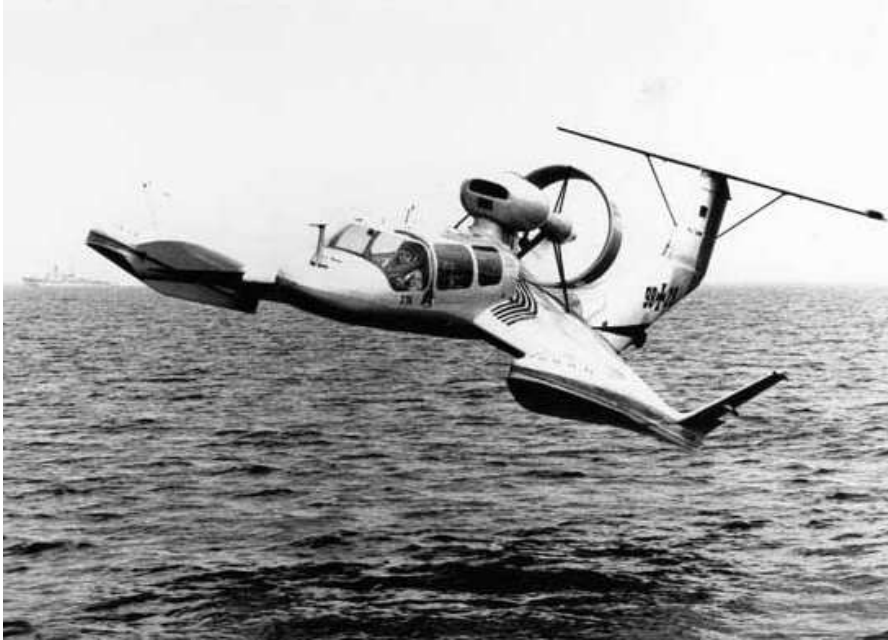
Figure 2.7: Lippisch's experimental WIGe vehicle, X-114
