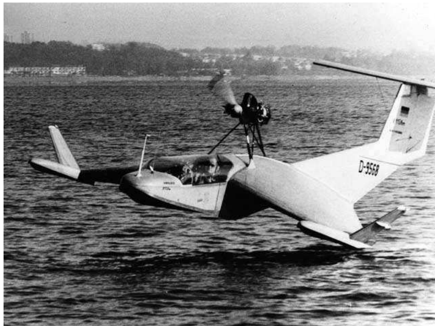
Figure 2.6: Lippisch's experimental WIGe vehicle, X-113
