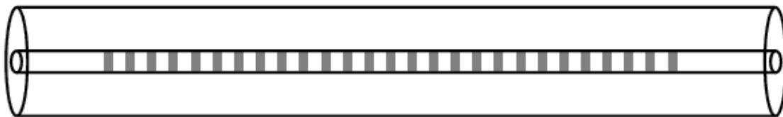
Figure 4.2: Structure of a uniform fibre Bragg grating
