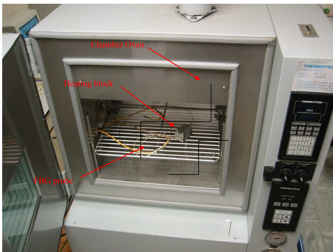
Figure 6.11: Experimental setup of the FBG based fire alarm system in Kidde PLC, UK
