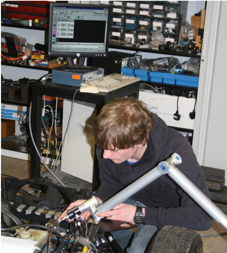
Figure 62 - The FARO Arm Coordinate Measurement Machine, used to measure the chassis and suspension mounting points of the RH2BP.
