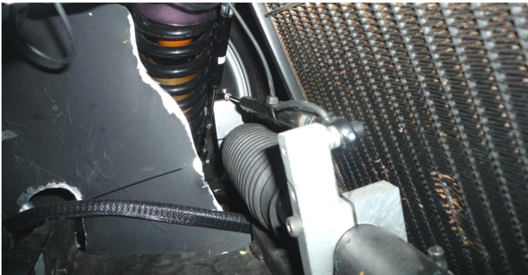
Figure 86 - The linear potentiometer mounted to the steering rack for measurement of steering angle.
