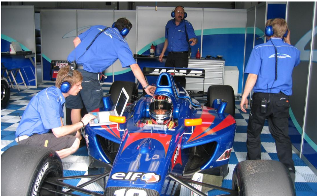
Figure 2 - The P1 Motorsport/Cram Competition team attend to Fairuz Fauzy's World Series by Renault car in the garage during a test session at Magny-Cours. This includes downloading and analysing recorded data, communicating with the driver and making setup changes.
