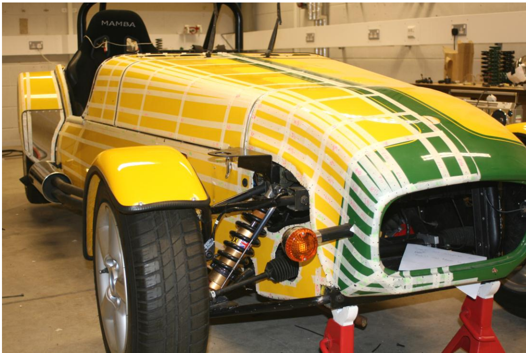
Figure 66 - Masking tape applied to the RH2BP bodywork. This allowed dot markers to be added to aid referencing of the photographs.
