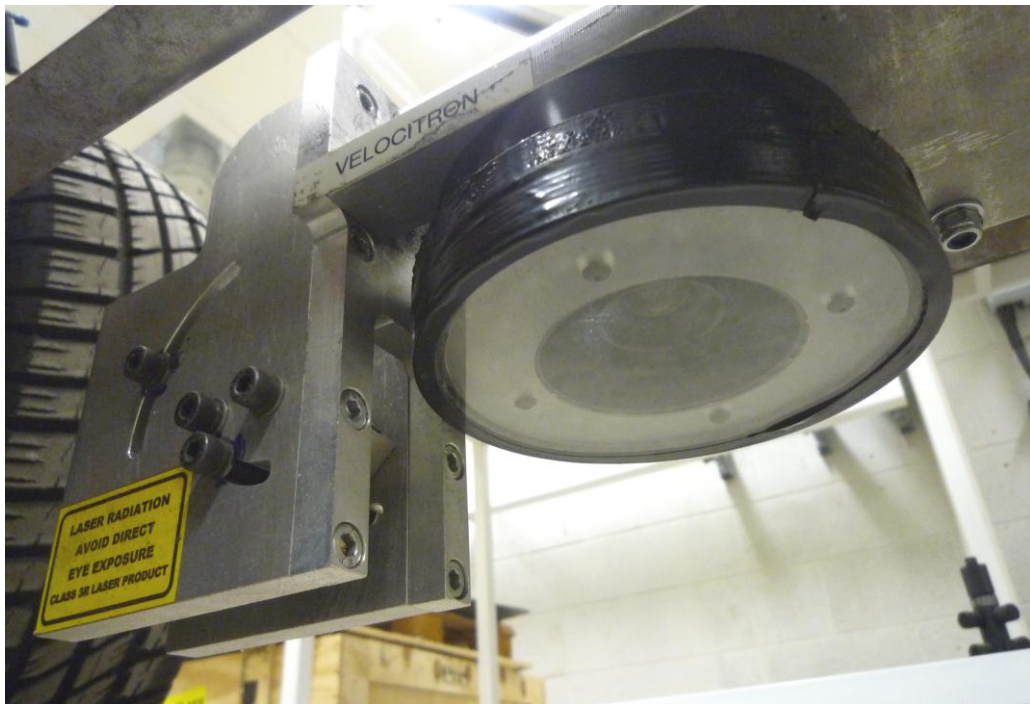
Figure 114 – Lens shield in situ over the LED light ring.
