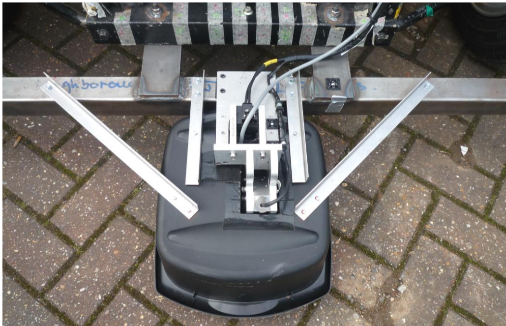
Figure 112 - The mounting of the ambient light shields.
