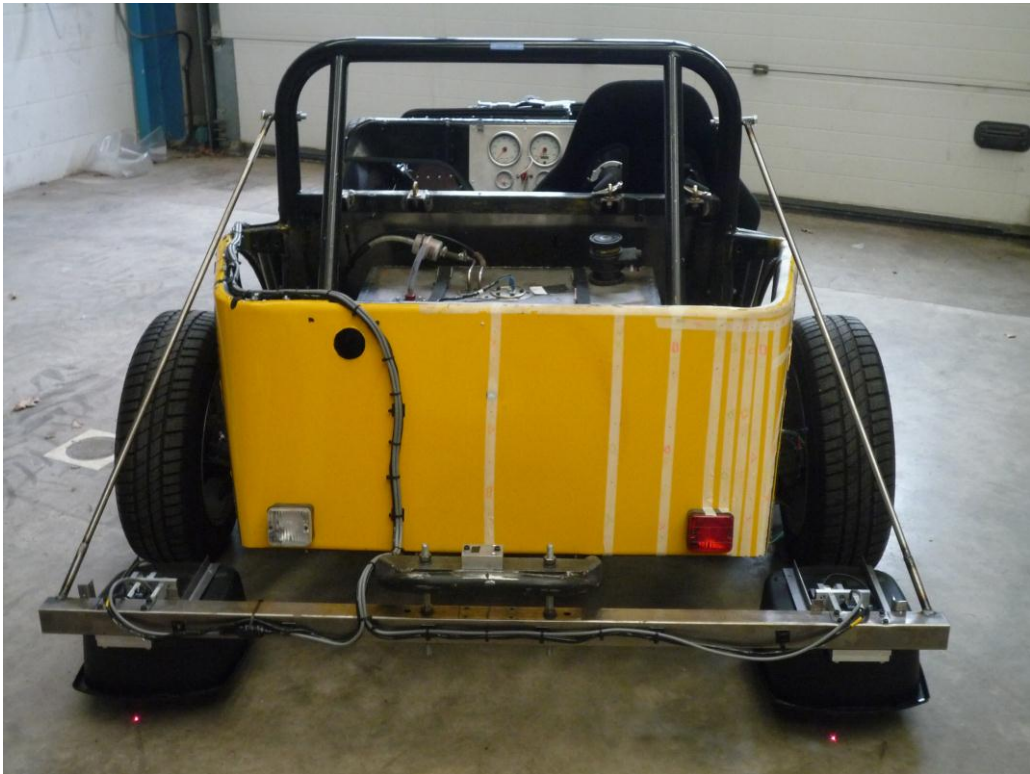
Figure 108 – The rear optical displacement/velocity sensor mounting beam.
