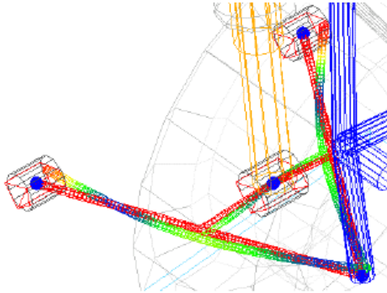
Figure 22 - Screenshot from ADAMS/Car showing the simulated deflection of the control arm or a suspension system.
