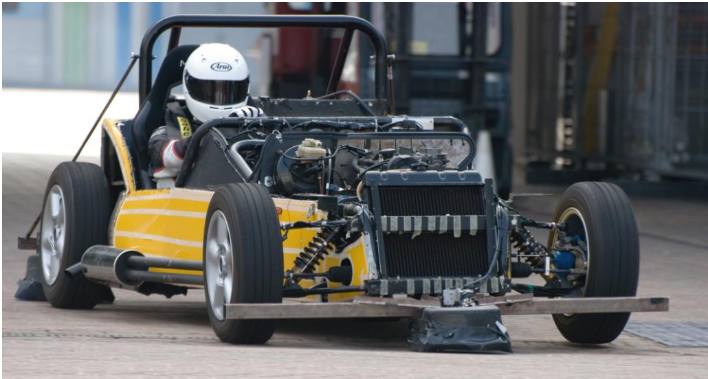
Figure 113 – The skirted ambient light shields in use during testing.
