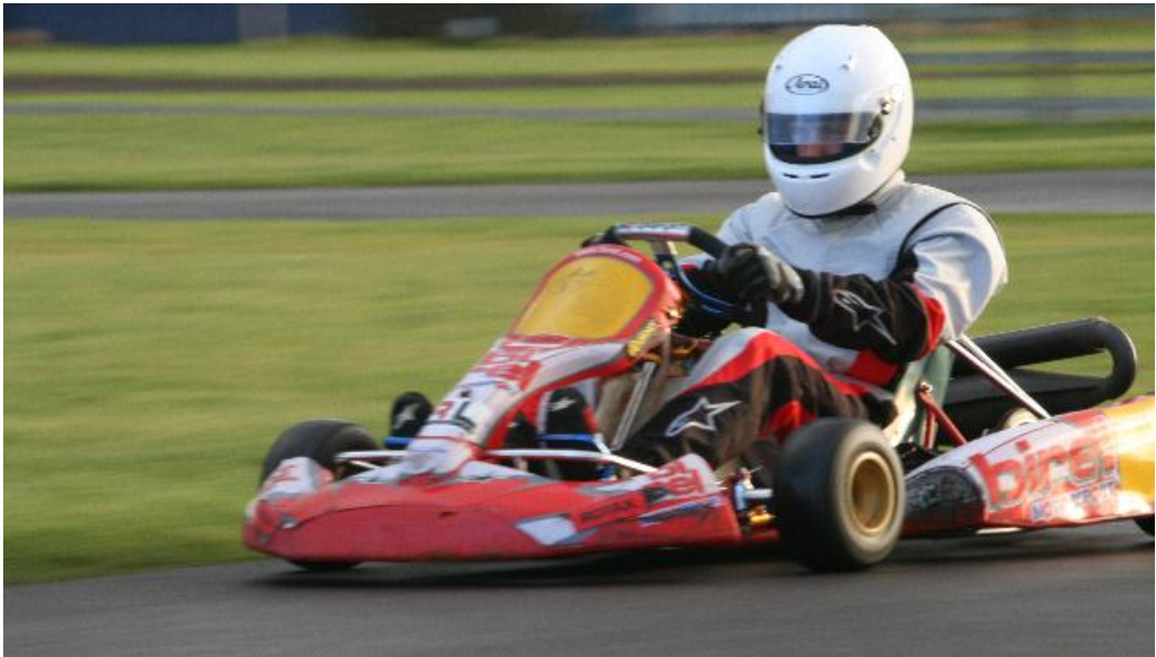
Figure 3 – A Rotax Max 125cc Two-stroke kart. Rotax Max is an extremely popular club, national and international kart class.
