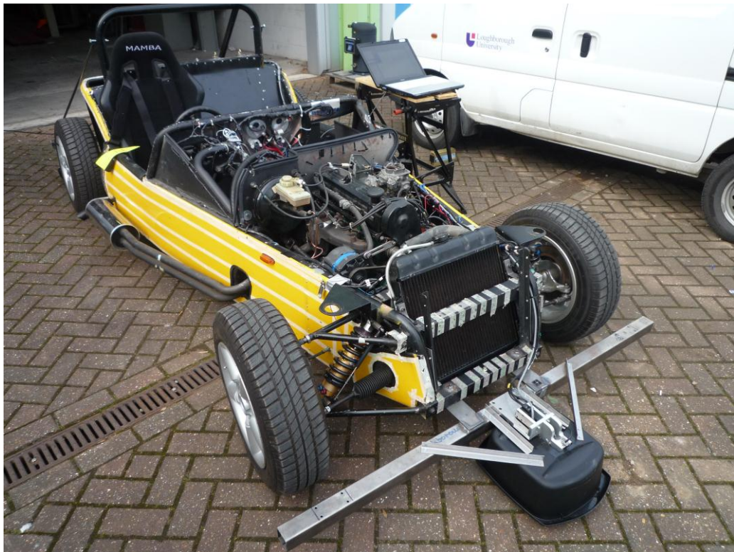
Figure 107 – The front displacement/velocity sensor mounting beam.
