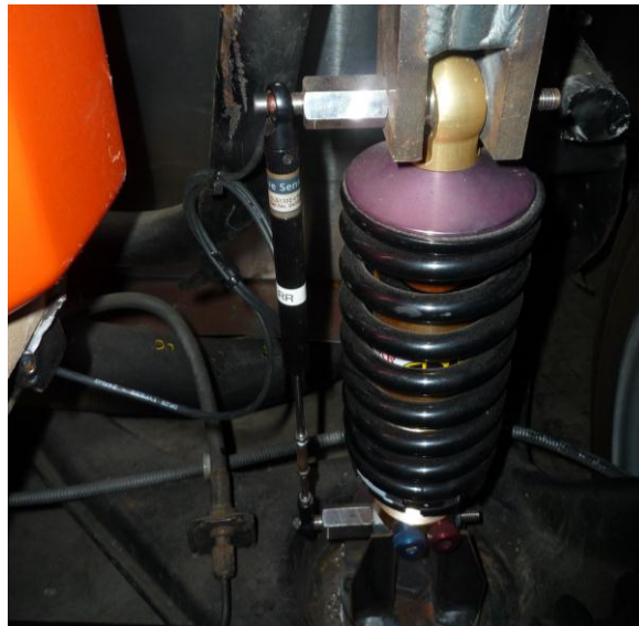
Figure 84 - Linear potentiometers mounted to the coil over damper units for measuring damper displacement/suspension deflection.
