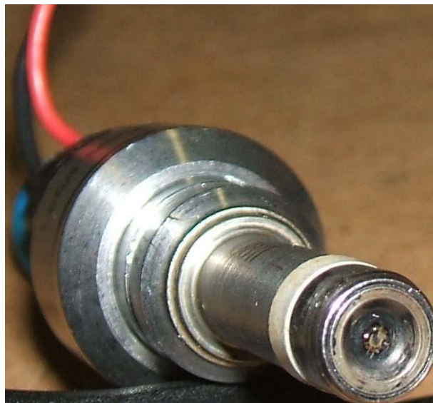
Figure 7.2: Injector 2: 6-hole 90° cone angle with a concave nozzle tip
