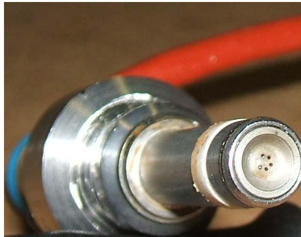
Figure 7.3: Injector 3: 6-hole 60° cone angle with a concave nozzle tip
