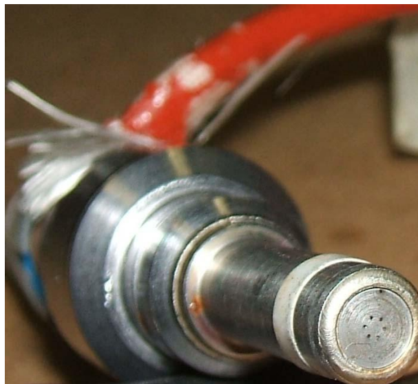
Figure 7.1: Injector 1: 6-hole 90° cone angle with a flat nozzle tip
