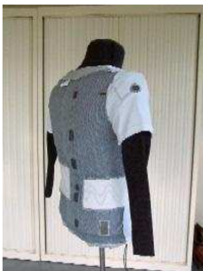
Figure 63: Telemetry ‘vest’ to monitor SFPs and Flight Crew
