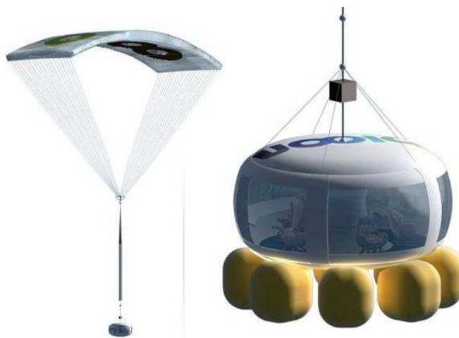
Figure 68: BLOON's 'Pod', Descent Aerofoil, Chain and Landing Sub-system
