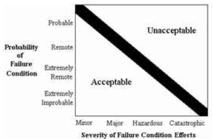
Figure 17: AC 25.1309 severity and probability criterion
