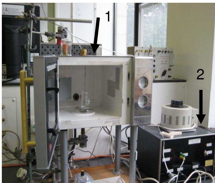
Figure 2.2.1.2 – Microwave and Control unit
