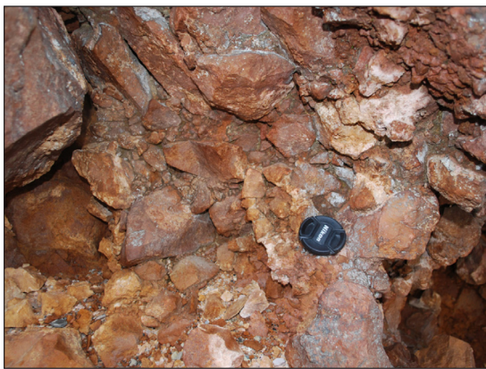
Fig. 4. E3. Lithofacies E is a poorly sorted clast supported breccia with a fine grained matrix.
