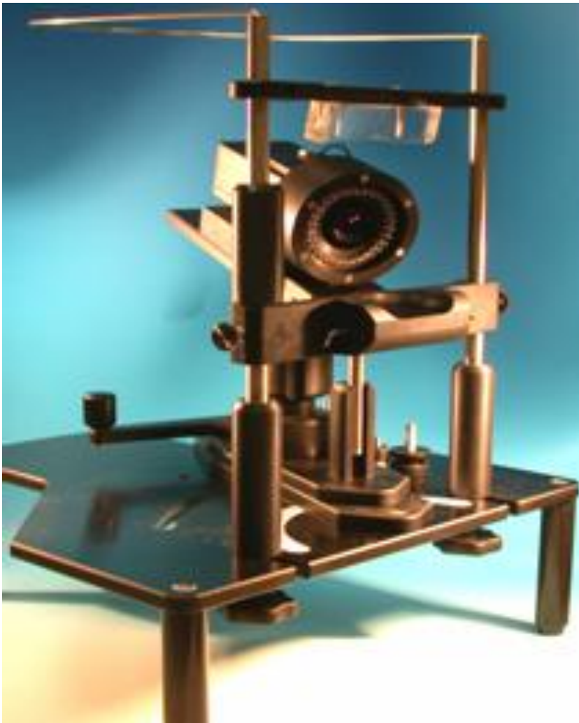
Figure 9.2. Image of bespoke QLF array together with geometry stabilizing equipment
