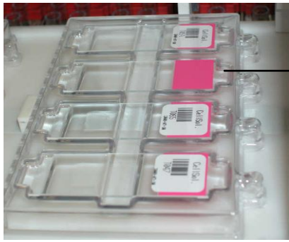
Figure 27: No label on the CS 120™ slide as the robotic arm failed to pick it up from the printer head
