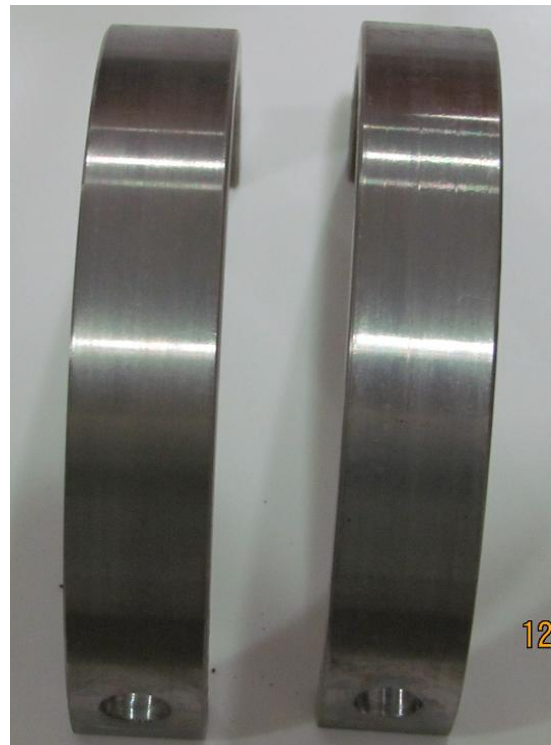
Test 4: 25Cr seawater 1000ppm NaNO 2 at 80°C
