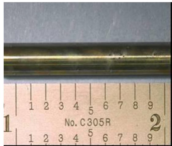
B: 13Cr 100ppm NaNO 3 at 80°C, 5ppb [O]
