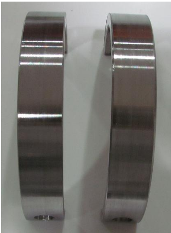
Test 3: 25Cr seawater 1000ppm NaNO 2 at 25°C
