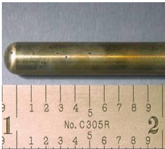
A: 13Cr blank solution at 80°C, 5ppb [O]
