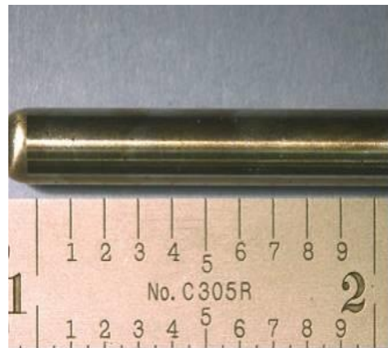
D: 13Cr deoxygenated solution 17ppb [O], with 100ppm NaNO 2
