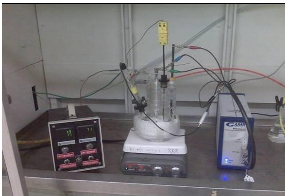
Figure 32: Figure showing the experimental setup of the glass cell
