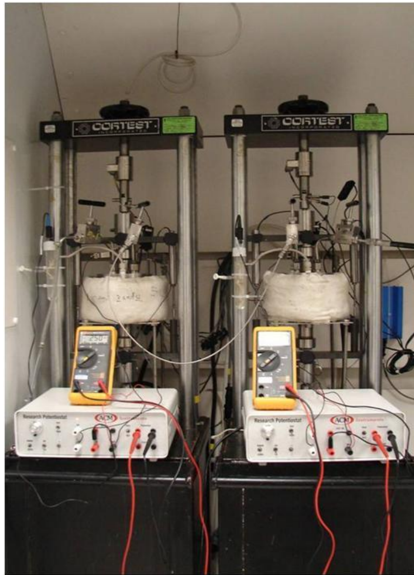
Figure 44: Picture of the SSR test setup
