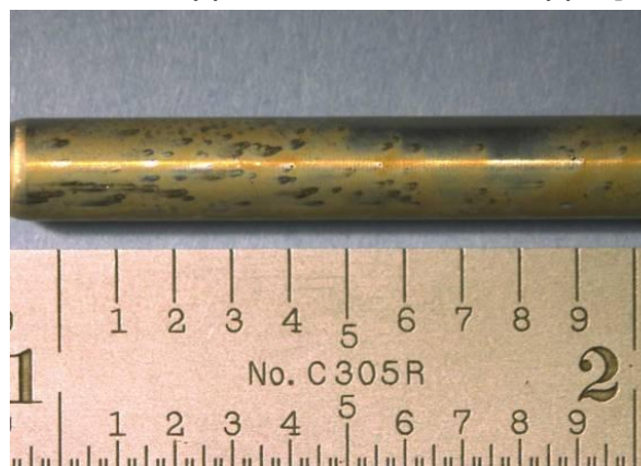
C: 22Cr 100ppm NaNO 2 at 80°C, 5ppb [O]
