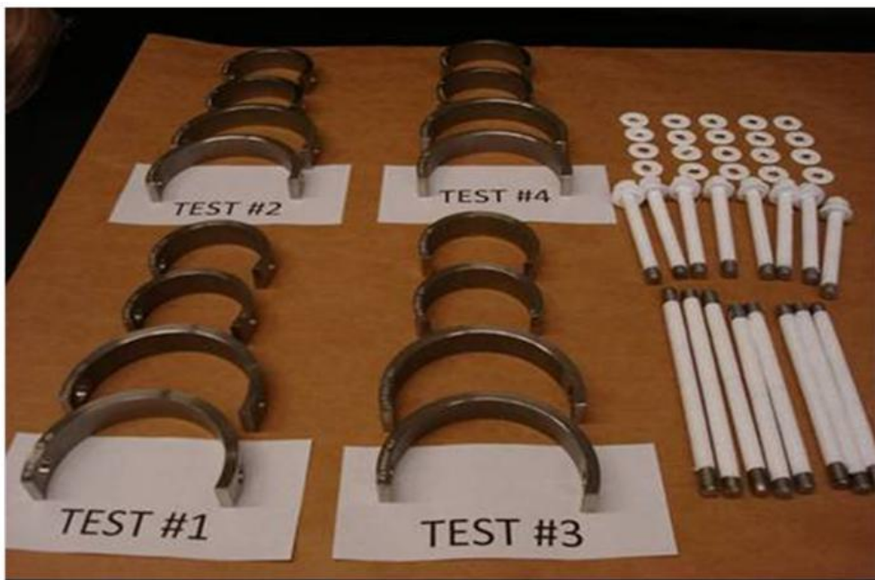
Figure 36: Picture of the C-rings and Teflon wrapped couplings before deflection
