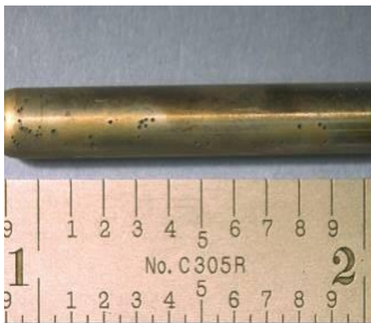
C: 13Cr 100ppm NaNO 2 at 80°C, 5ppb [O]
