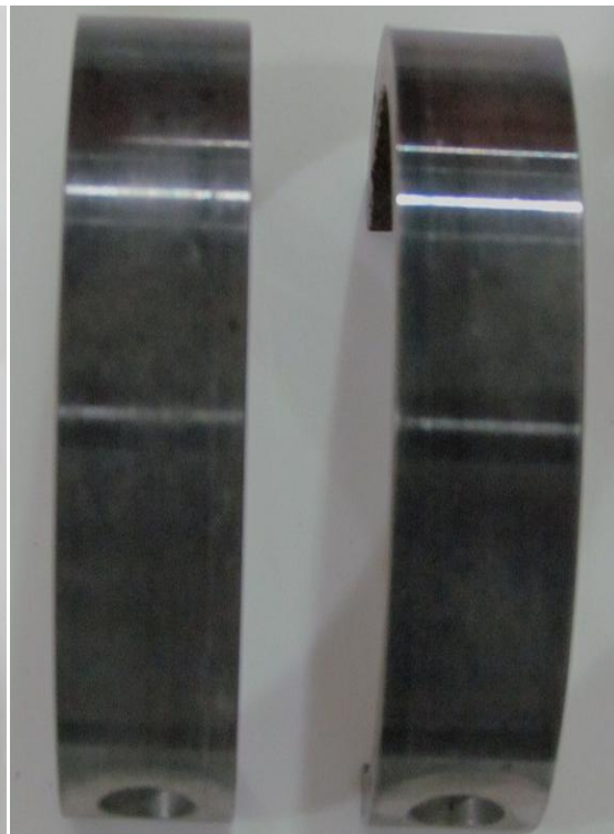
Test 4: 13Cr seawater 1000ppm NaNO 2 at 80°C
