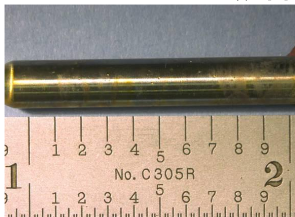
B: 22Cr 100ppm NaNO 3 at 80°C, 5ppb [O]
