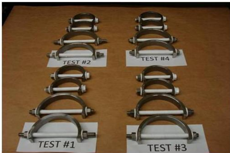
Figure 38: Picture of the C-rings after deflection
