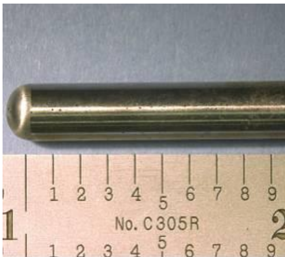
C: 13Cr deoxygenated solution 17ppb [O], with 100ppm NaNO 3 at 25°C
