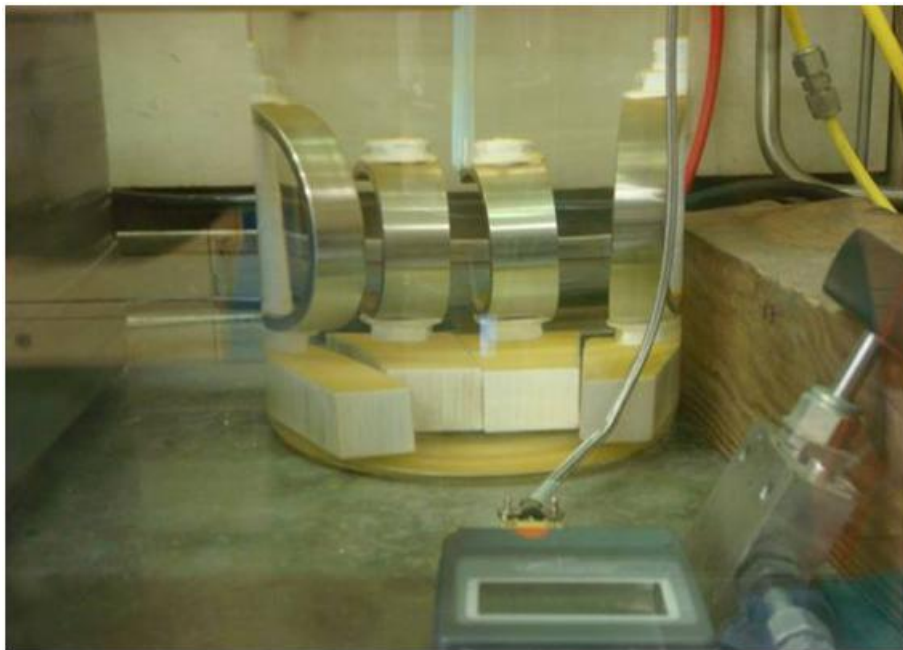
Figure 41: Picture showing close up of the 4 C-rings in a glass autoclave
