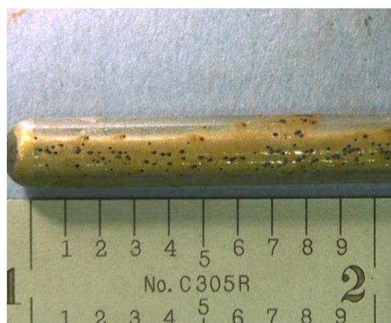
D: 13Cr 400ppm NaNO 2 at 80°C, 5ppb [O]
