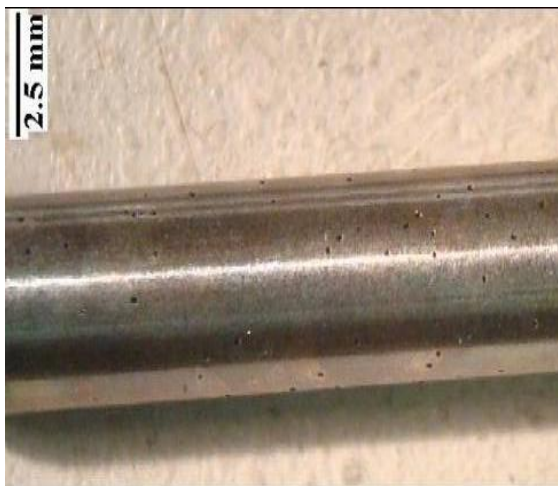
A: 13Cr fully oxygenated blank solution, 7600ppb [O] at 25°C
