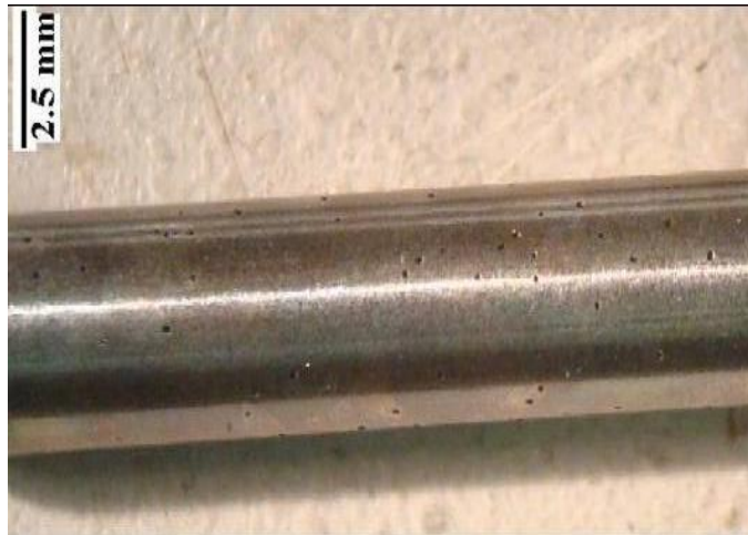
A: 13Cr fully oxygenated, 7600ppb blank at 25°C
