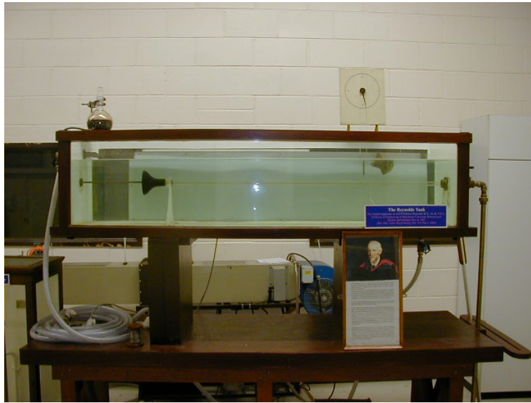
Figure 1.1: Reynolds' tank for the experiment about transition from laminar to turbulent flow
