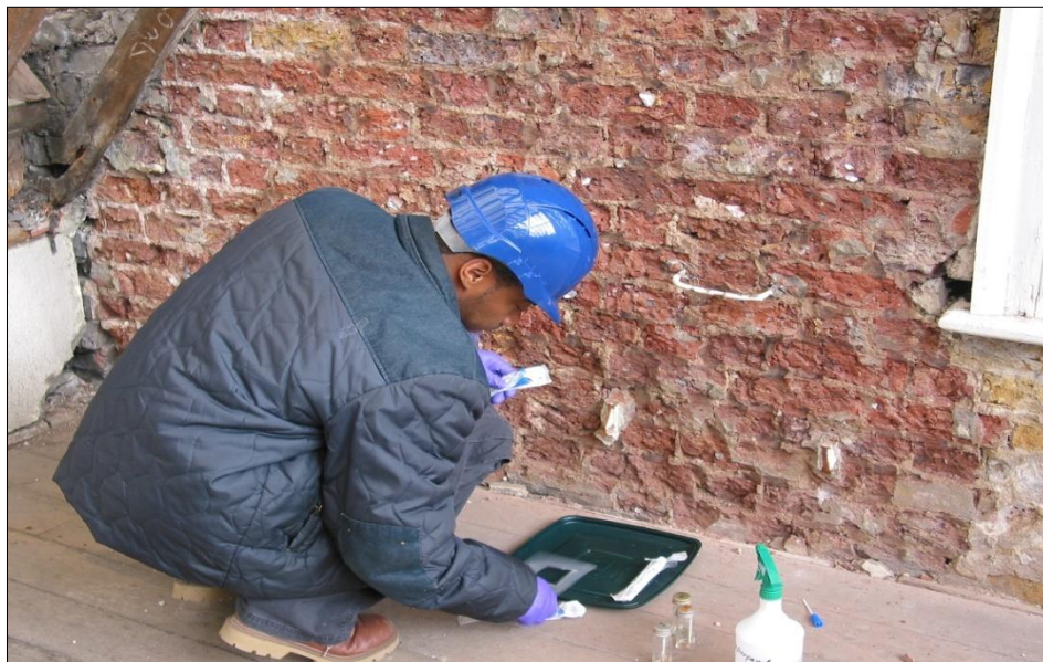
Plate 2.1 Swab sampling in progress at BRE Victorian stable block, Watford
