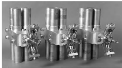
Figure 8.15 The Johnson Matthey HotSpot™ reactor. These can be made in different forms suitable for methanol, methane, or gasoline processing. (Picture by kind permission of Johnson Matthey plc.)
