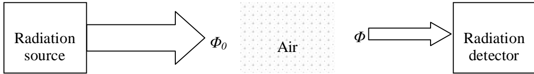
Figure 3.4: Schematic diagram illustrating the operating principles of the IRGA.
