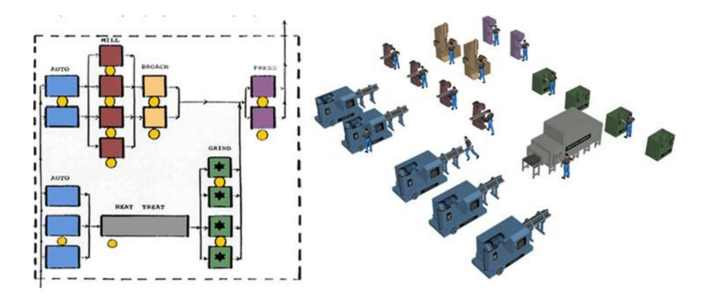
Figure 7-1: The Initial Factory Layout and the 3D Mock-Up of the Spindle Assembly Cell
