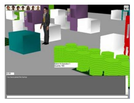
The Virtual World client interprets the data received from the Virtual World server and translates them into graphics. For example, the number of raw material is translated into blocks as illustrated in the above figure. If there is an issue in the process, the user can detect it easily.
