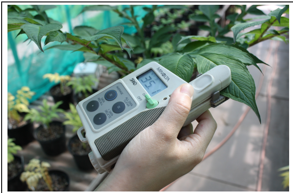
Plate 2.4 Minolta SPAD-502 meter for determination of relative chlorophyll content. Whilst taking measurements of relative chlorophyll content, the head (composed of an IR source and detector) was closed to enclose the leaf material being analysed.
