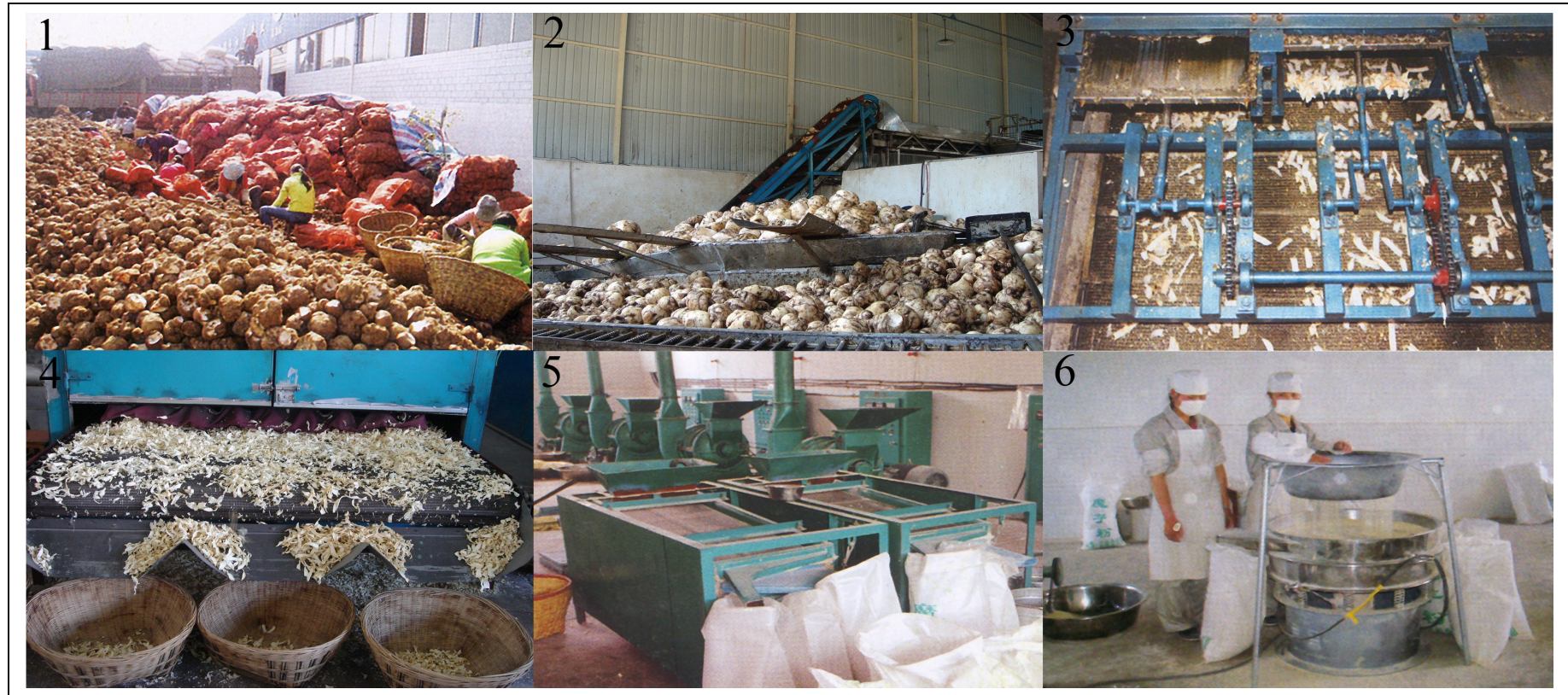
Figure 1.10 Various stages of the production of “common konjac flour” from fresh corms. Photographs taken during a personal visit to Fuyuan Golden Field Agricultural Products Company Ltd, Yunnan Province, P.R. China in November 2008. (1) Selection of disease-free corms for flour production. (2) The corms are transported to a washing apparatus by conveyer belts and are washed to remove dirt and soil. (3) The corms are sliced into chips of 2 - 3 mm in thickness. (4) The fresh chips are dried in a hot air drier to remove moisture. (5) The dried chips are milled to produce crude konjac flour. (6) Removal of micro-fine powder ( i.e. impurities) from the crude flour via sieving.
