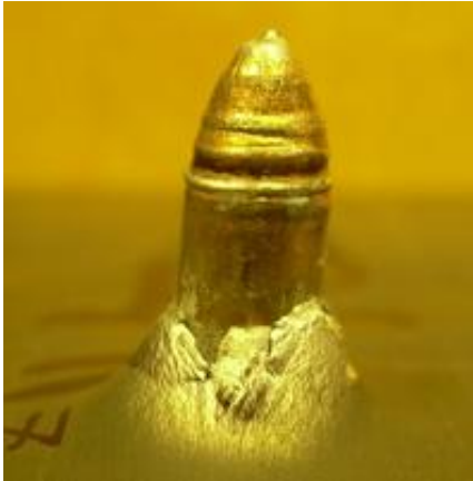
Fig.7a. Armour piercing (AP) partial penetration. b. Fragment simulation projectile (FSP) (Courtesy Cranfield Shrivenham)
