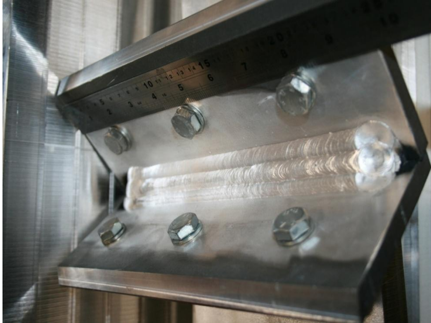
Fig 48. Welded crack test sample – 12.7 mm thick material.
