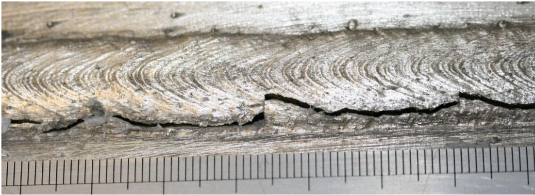
Fig F3. Weld solidification cracking in 7xxx base material resulting from uncontrolled Zn mixing using three wire system (Al-Zn-Mg weld composition)
