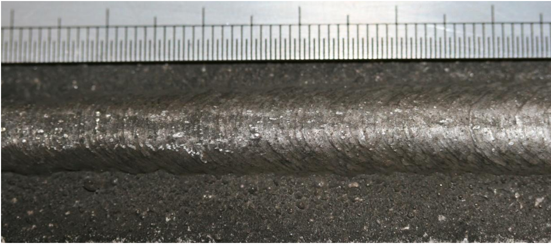
Fig F1. Weld deposited using Al-5039 filler showing heavy sooting / tenacious crust on weld and Al-1100 base material.
