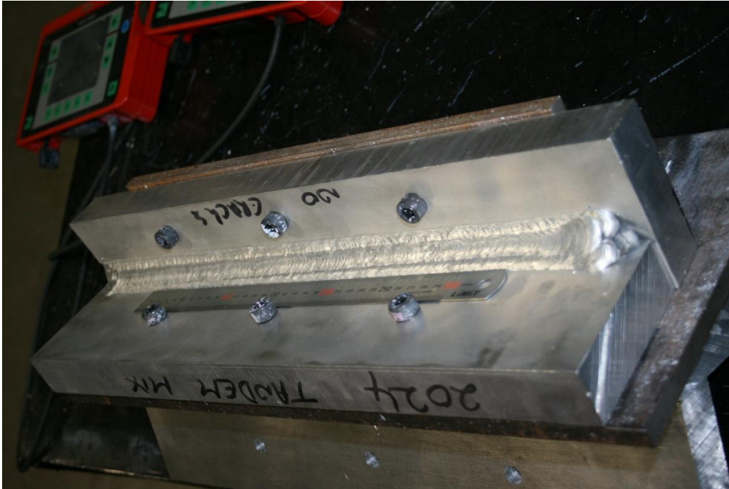
Fig 50 thick crack sample (30 mm)
