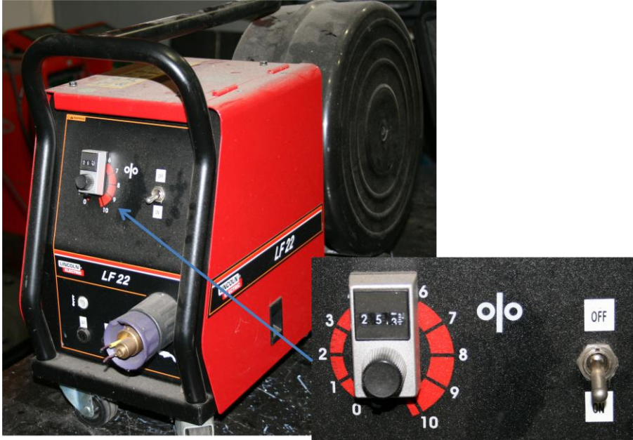
Fig 34. Lincoln Electric LF22 cold wire feed unit showing analogue wire feed control and manual trigger on/off (inset).
