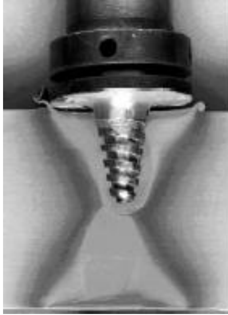
Fig 11. Whorl™ tool geometry and 75 mm thick double pass joint (TWI Ltd)
