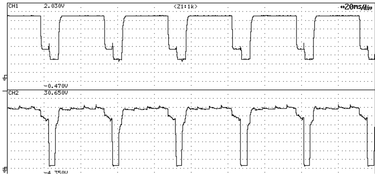
Fig B3. Arc length correction +10 Readings V_{MAX} 24.9 \text{ V} ; P_i 2700 \text{ W} ; W_f \sim 6.4 \text{ m min}^{-1}
