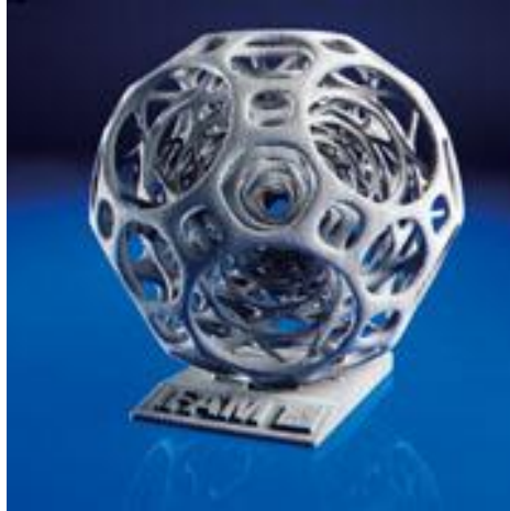
Figure 20: A model with complex shape created by Rapid Prototyping [Fraunhofer 2007]
