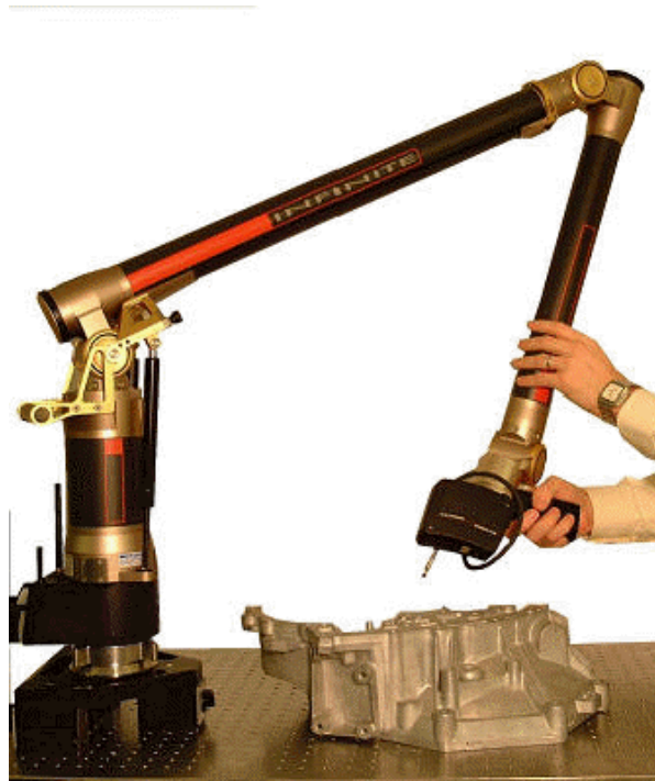
Figure 33: A type of portable 3D laser scanner [Nvision3d 2007]
