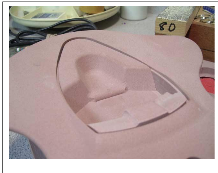
Figure 19: A model with high surface quality created by CNC machining [product design forums 2005]
