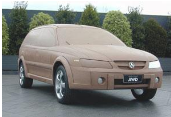
Figure 11: The full-scale clay model of a car design [car design online 2011]
