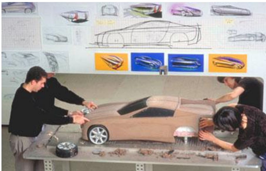
Figure 10: The small scale clay model of a car design [car design online 2011]
