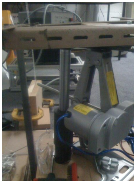
Figure 51: Electrical car jack
