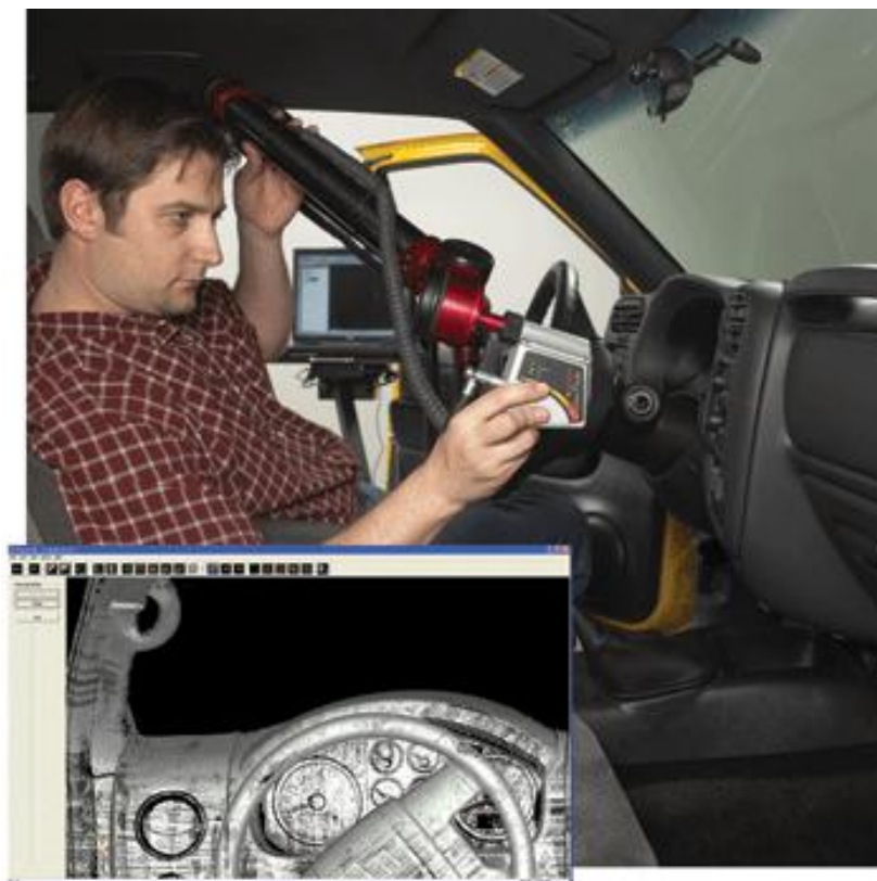
Figure 26: The use of 3D scanning in creating a virtual prototype [T&P 2007]
