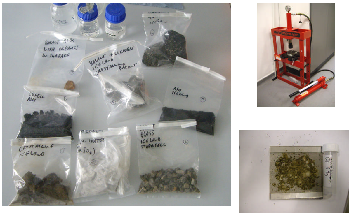
Figure 4-16: Photographs illustrating processing of analogue samples (left) unprocessed analogue samples supplied by Prof. Charles Cockell, (top right) 10 tonne hydraulic press used for crushing samples in preparation for liquid extraction (bottom right) analogue sample after crushing on stainless steel plate with 1 mm spacers.
