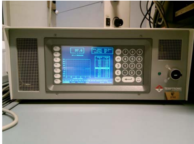
Figure 3.5: The temperature control facility.
