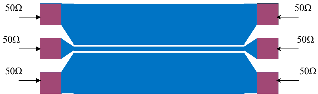
Figure 3.17: Simulation setup using single port definition used in eliminating higher order modes in EM simulations.
