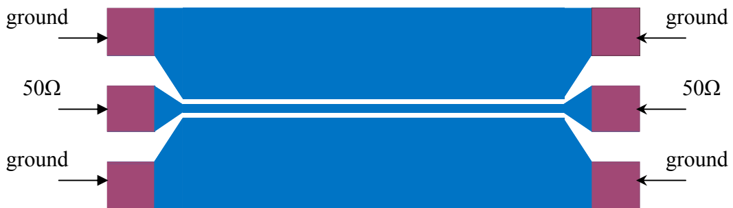
Figure 3.16: Conventional setup used in the measurement and simulation of a CPW line, with a length of 1.4mm.
