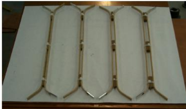
Figure 2-28 Coil-to-coil electrodes used for lightning impulse tests with solid interface at gap distances from 3 mm to 12 mm [75].
