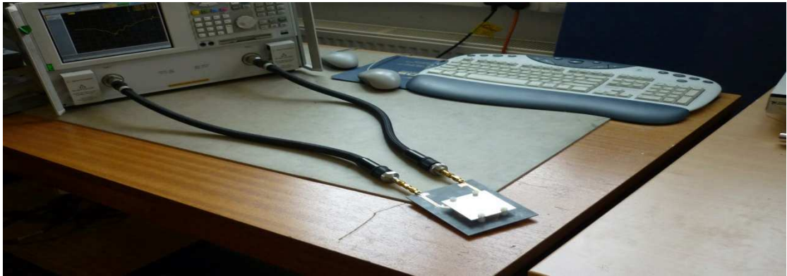
Fig.8.1: Experiment to determine return loss and isolation of single element
