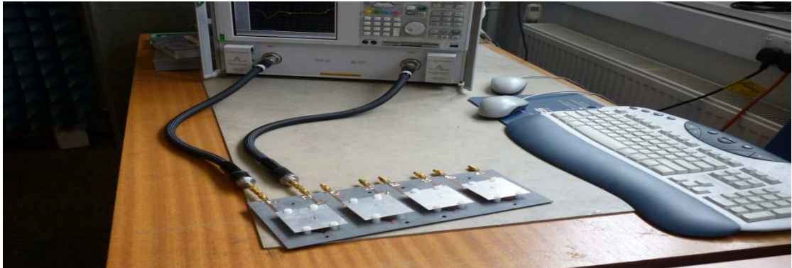
Fig.8.4: Experiment to determine return loss and isolation of 4 array antenna
