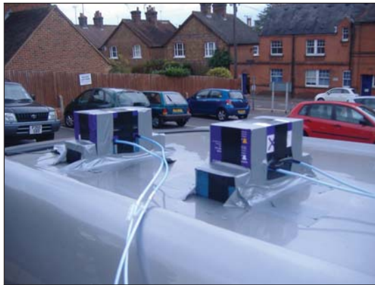
Figure 6.13: Photograph of the receive antennas used in Bishops Court measurement.
