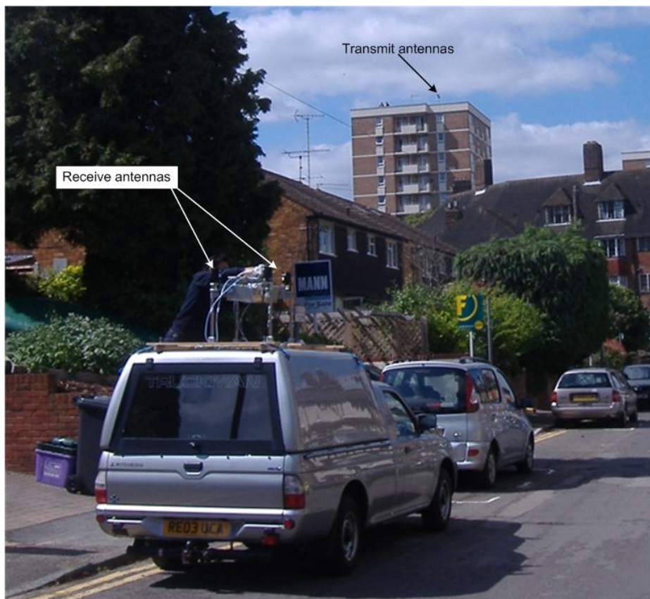
Figure 4.11: Pictorial view of tower block mounted emulated satellite transmitter and vehicular mobile receiver
