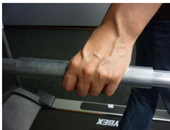
FIGURE 4.3: SLIDING HANDRAILS ALLOW NATURAL FREE MOVEMENT OF THE ARMS WHILST STILL PROVIDING STABILITY
