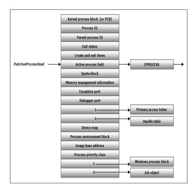
Figure 2.5 Structure of an EPROCESS block<sup>6</sup>
