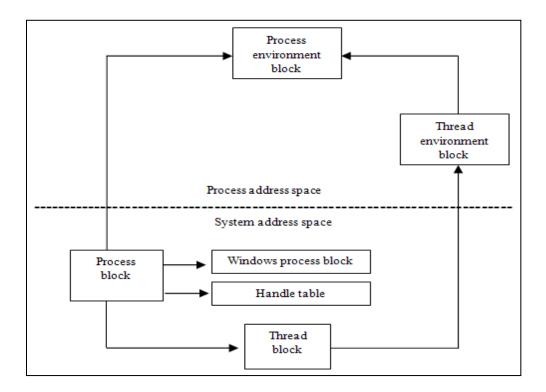
Figure 2.4 Data structures associated with process and threads<sup>5</sup>
