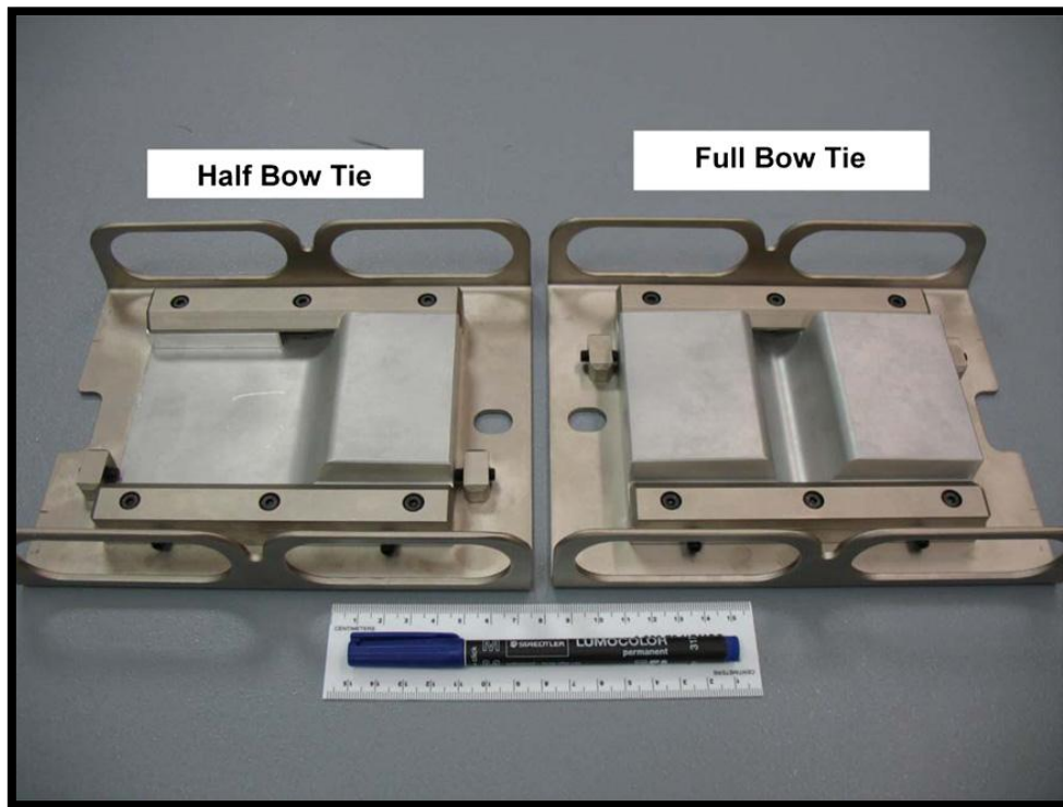
Figure 7: Full and half bow-tie filter used in the Varian OBI v1.4 (Ding et. al., 2007).
