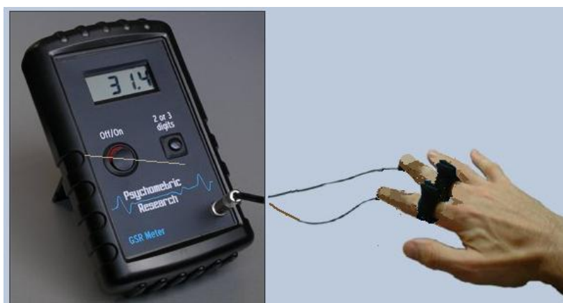
Figure 5.1: The GSR Meter and its electrodes attaching position with hand as used in the experiment. The output shows a measurement of 31.4 micro Siemens ( \mu\text{S} )
