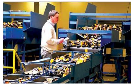
A Kodak employee inspects inbound cameras at the firm's primary recycling facility in Rochester, New York. Vibrating tables sort the cameras by model.
